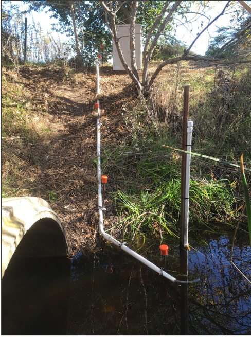
Infrastructure for automated ISCO samplers at Whittier stormdrain outflow (left) and Phelps Creek (right).
