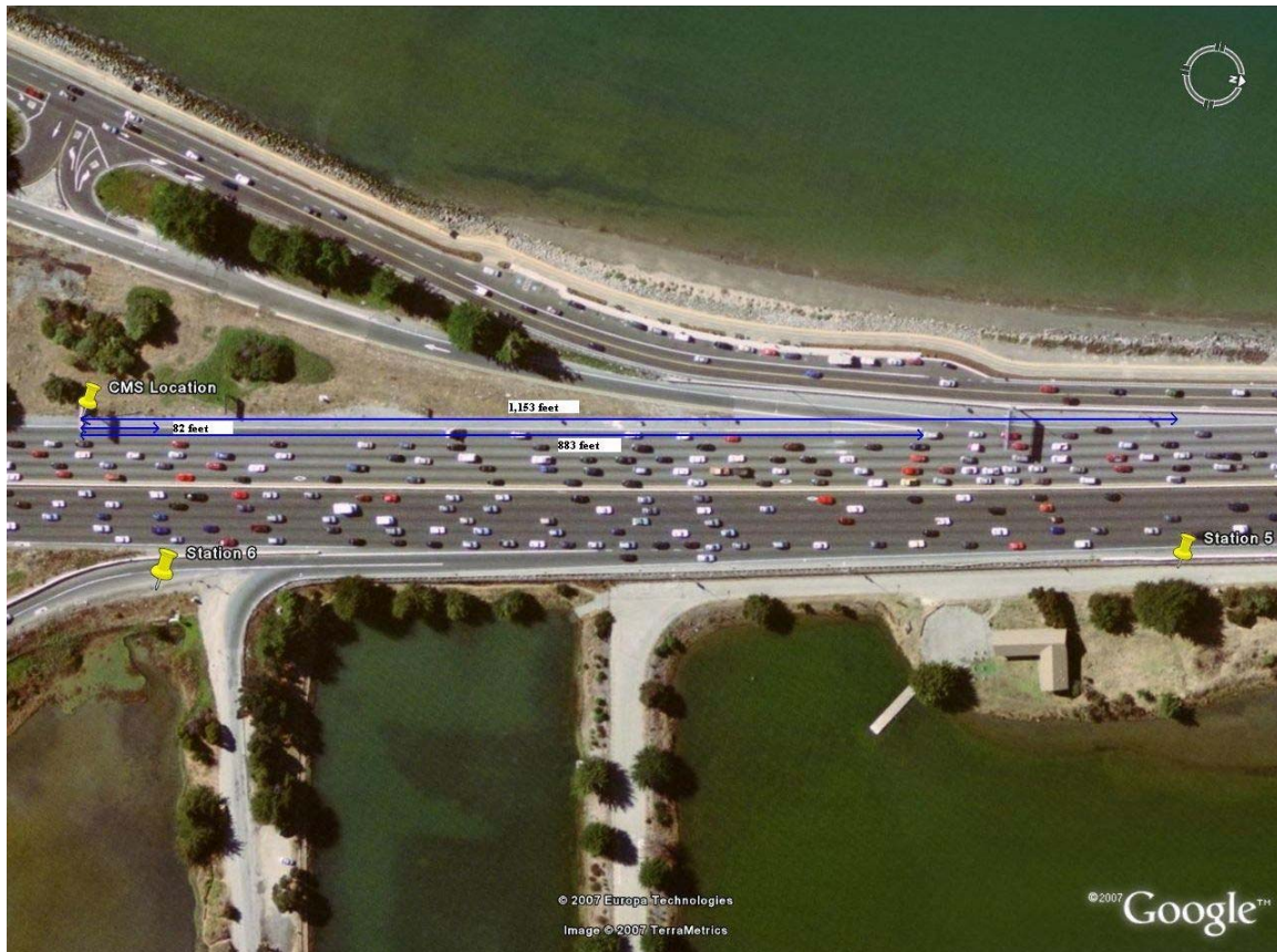
Figure 5: The line of loop detectors at station 6 are estimated to be around 80 feet “upstream” of the CMS, while those of station 5 are around 1,150 feet “upstream” of the CMS. The sign and stations are marked with superimposed yellow thumbtacks.
