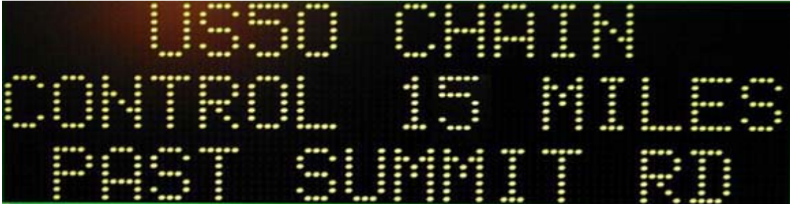
Figure 10C: The second frame of a two-frame CMS message with the '3' changing to a '5'. The frame is left on for 1 second.
