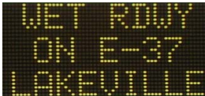
Figure 11B: The first frame of a two-frame CMS that is compacted. The frame is left on for 1 second.
