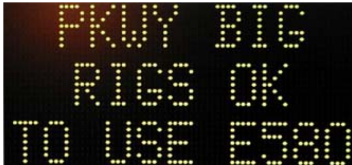
Figure 7C: The 2 nd frame of a two-frame CMS message. The exposure duration is 1 second.
