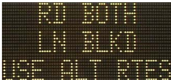
Figure 11C: The second frame of a two-frame CMS that is compacted. The frame is left on for 1 second.
