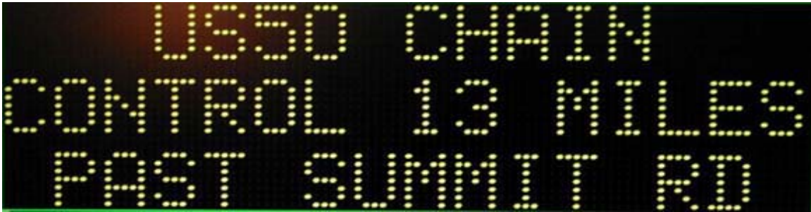
Figure 10A: The first frame of a two-frame CMS message. The frame is left on for 1 second.
