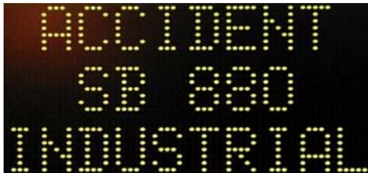
Figure 7A: The first frame in a two frame portable CMS sign left on for a duration of 1 second.
