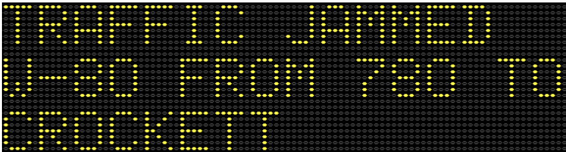
Figure 8A: The permanent CMS sign for traffic information is left-justified (LJ).
