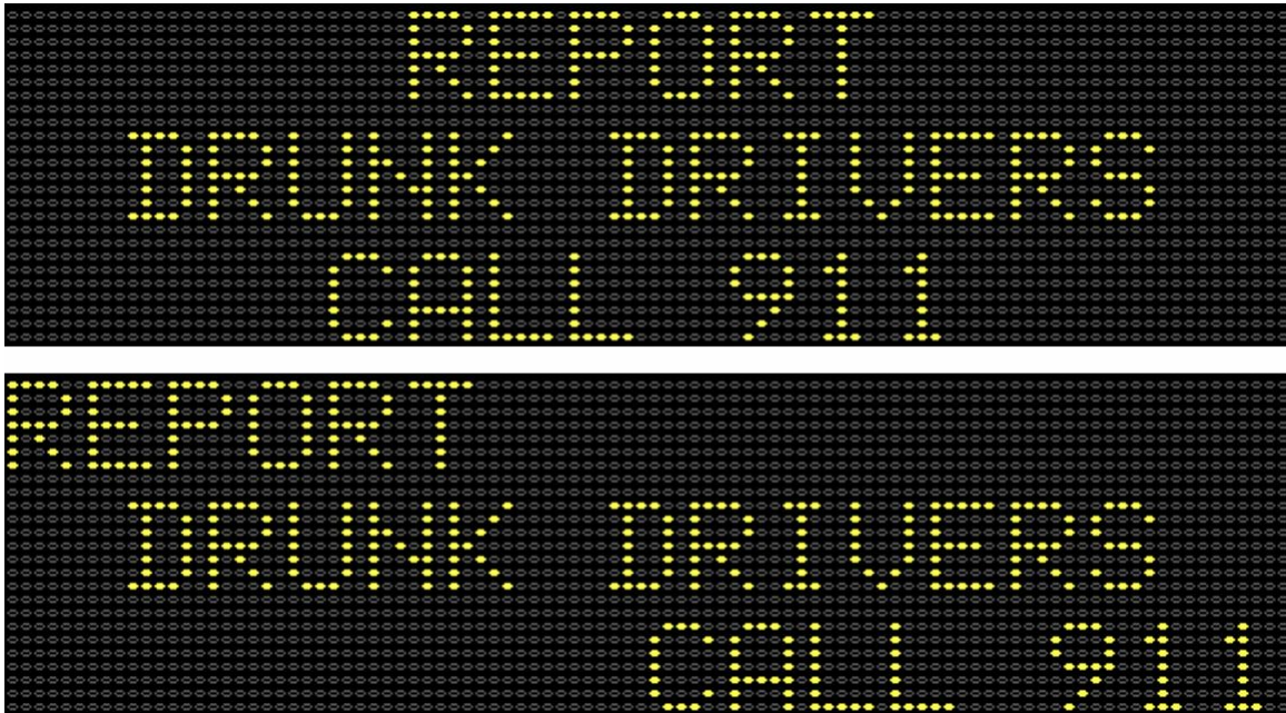
Figure 6: Shown here are the standard configuration – center justified (upper message) and the test configuration – staircase justified (lower message). Although the content of each message is identical and only the configurations are different, they will be referred to as the “standard message” and “test message” for simplicity.
