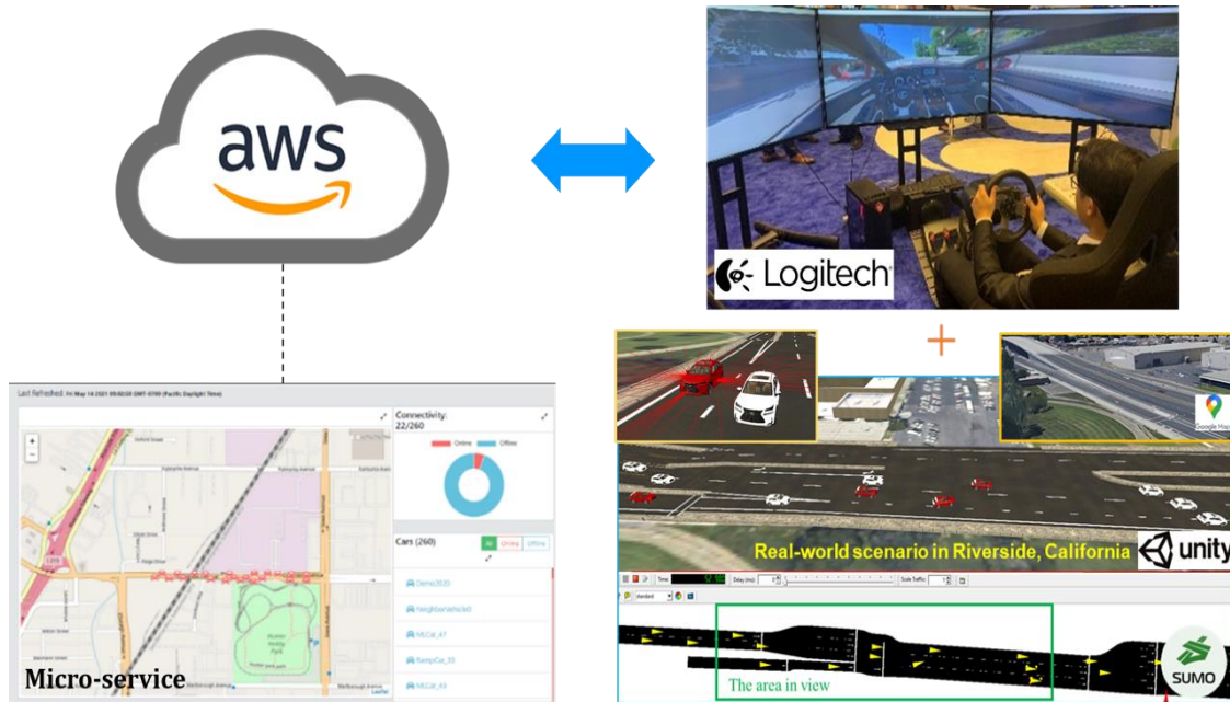
Fig. 4-3 Human-in-the-Loop Unity-SUMO co-simulation based on a real-world ramp merging area in Riverside, CA
