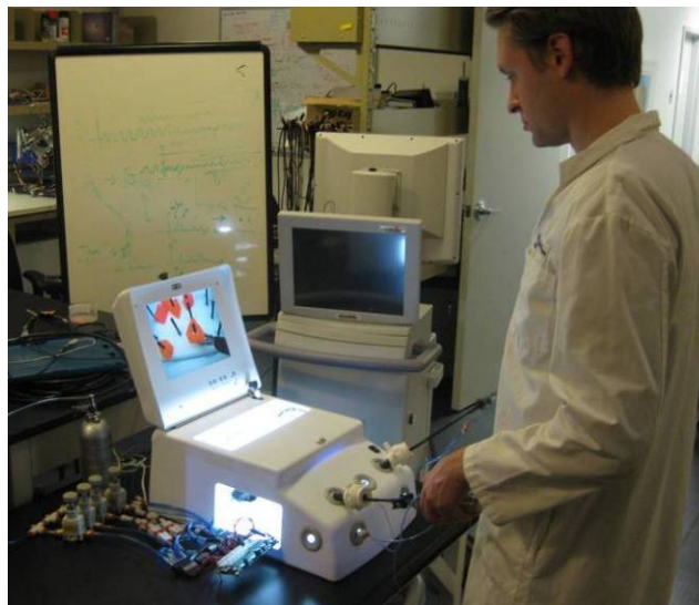
Figure 59. Tactile Feedback system integrated into a non-robotic laparoscopic grasper.
