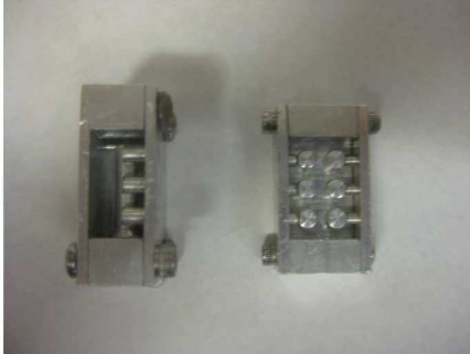
Figure 34. (Left) Single-Tube actuator mold for laparoscopic surgery (Right) Six-Tube actuator mold for remote and robotic surgery
