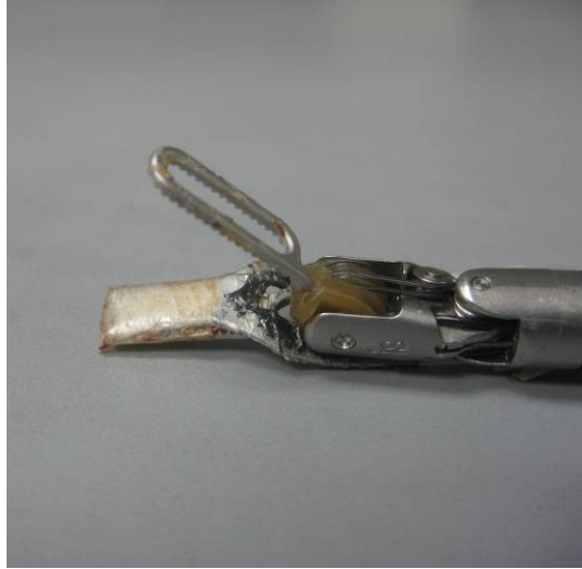
Figure 62. Waterproof sensor mounted on robotic grasper
