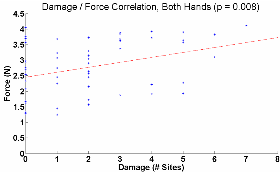
Figure 82. Correlation analysis of damage and mean grasping force.
