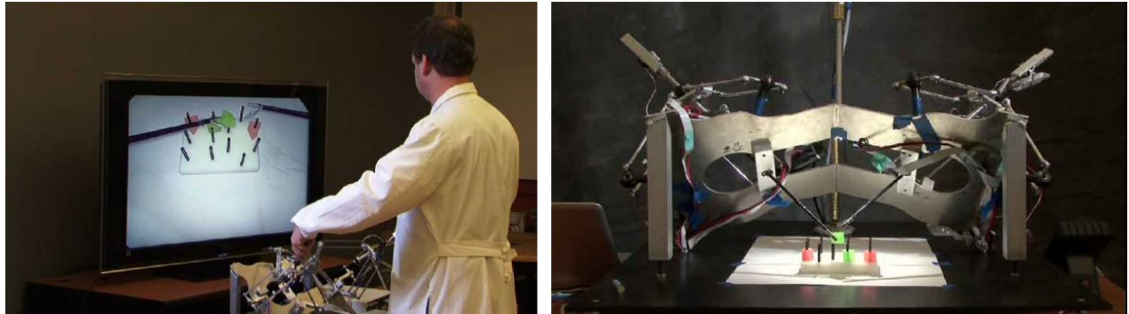
Figure 103. (Left) The LapaRobot Control Station allows the surgeon to tele-operate using standard laparoscopic instruments in a conventional arrangement. (Right) The surgical robot is operated to perform the training task.
