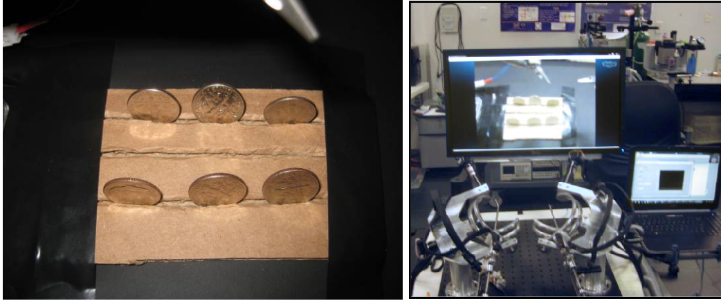
Figure 116. (Left) Subjects used the LapaRaven to retrieve six vertically mounted dimes. (Right) Perspective from the LapaRobot Master.
