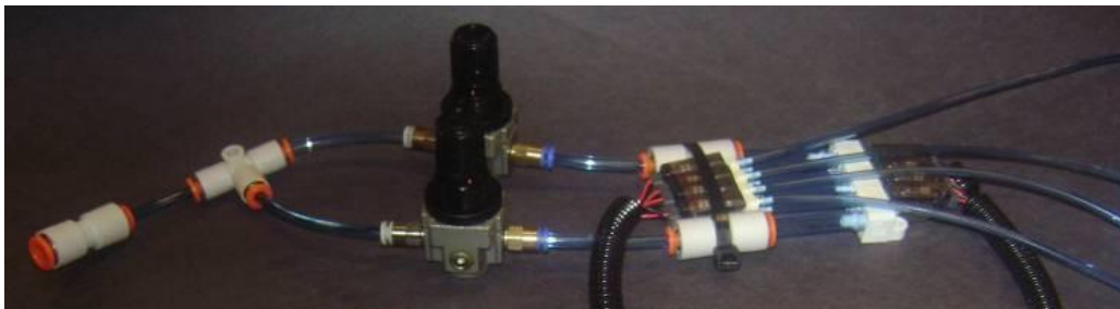
Figure 36. Three-Level Valve Pneumatic System
