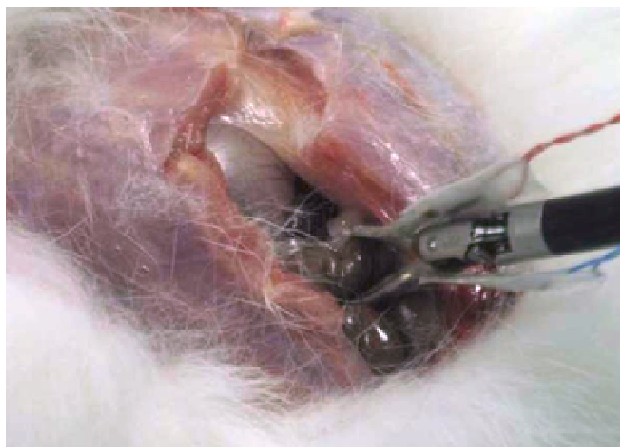
Figure 28. (Left) Sensor-equipped graspers on tissue in a leporine cadaver. (Right) Grip force recordings.
