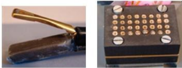
Figure 11. The grasper mounted sensor and motor driven tactile display by Ottermo et. al.
