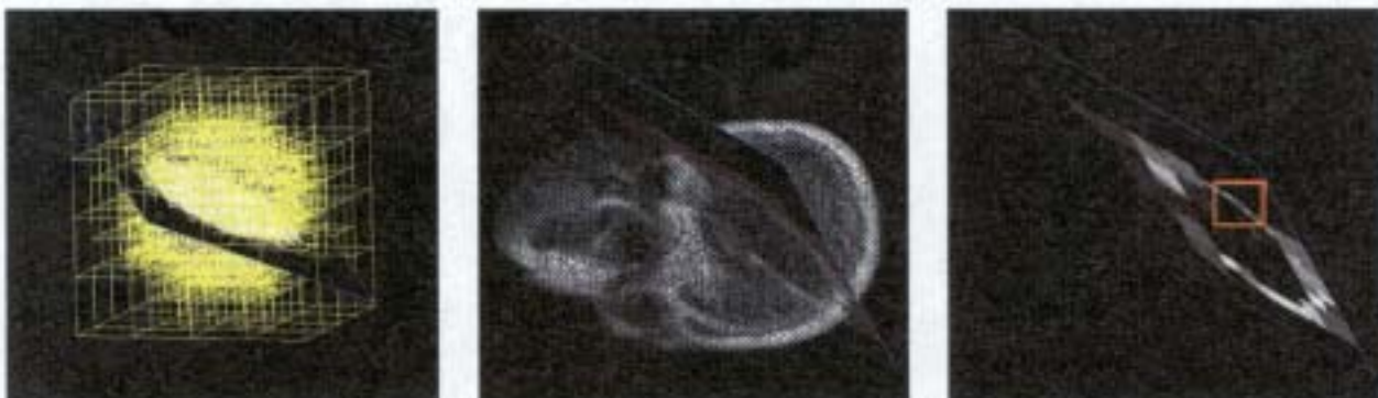
Cutting Plane through Sphere and Skull Data Sets. Red Polygon is ROI
