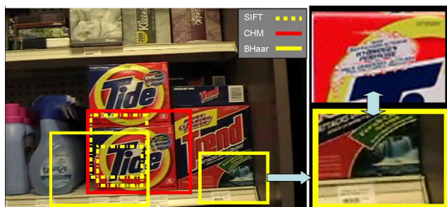
Figure 10. Example of good localization performance by all the methods for product 34. The in vitro image detail on the top right resembles the only false positive.
