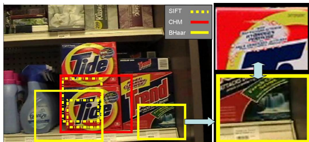
Figure 10. Example of good localization performance by all the methods for product 34. The in vitro image detail on the top right resembles the only false positive.
