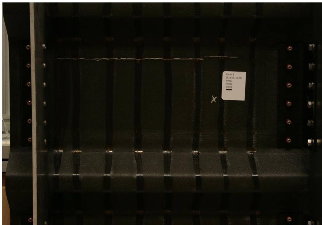
Figure 76. Type I: Back of SP021 (445.0 J), SP022 (540.0 J), and SP023 (665.5 J).
