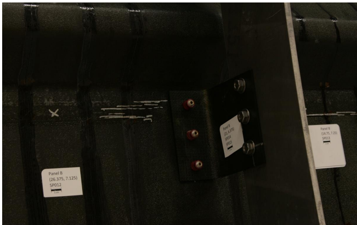
Figure 66. Type IV: Back of SP014 (348.0 J) and SP015 (728.0J).
