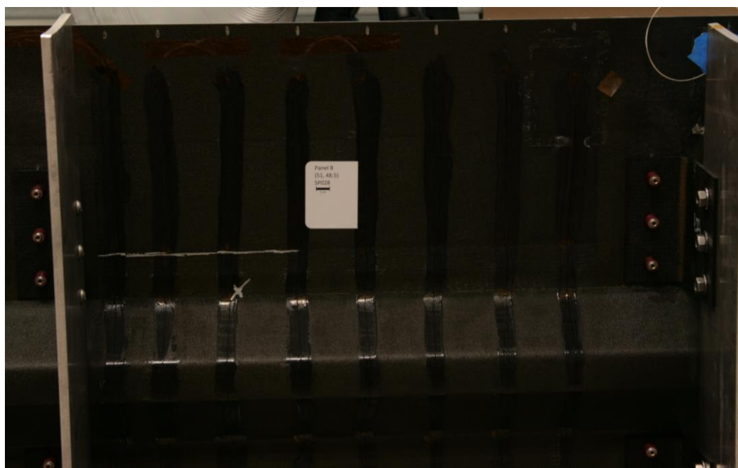
Figure 83. Type IIb: Back of SP028 (383.4 J).
