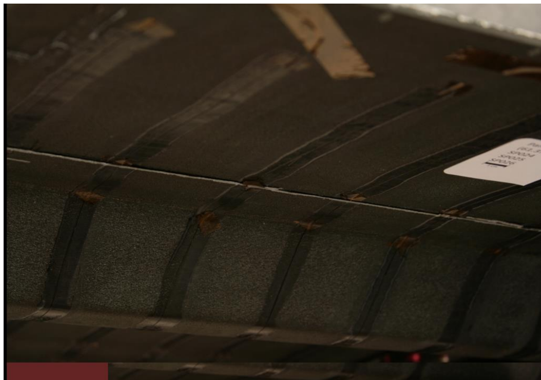
Figure 79. Type I: Unzipping of Flange at Location of Back of SP024 (432.9 J), SP025 (550.2 J), and SP026 (734.8 J).
