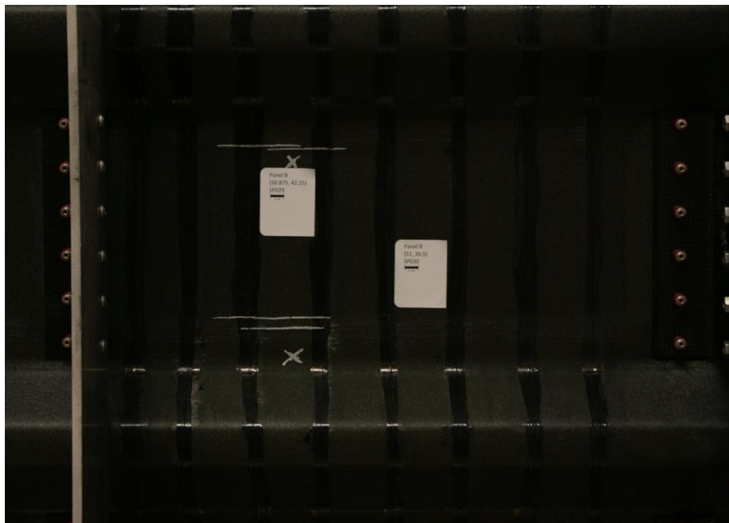
Figure 85. Type IIa: Back of SP029 (423.3 J) and SP030 (407.9 J).
