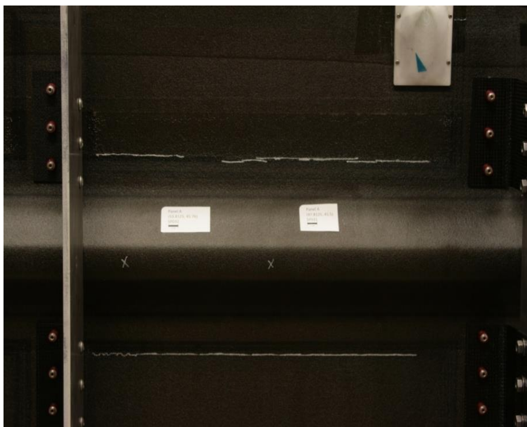
Figure 87. Type III: Back of SP031 (394.8 J) and SP032 (560.8 J).
