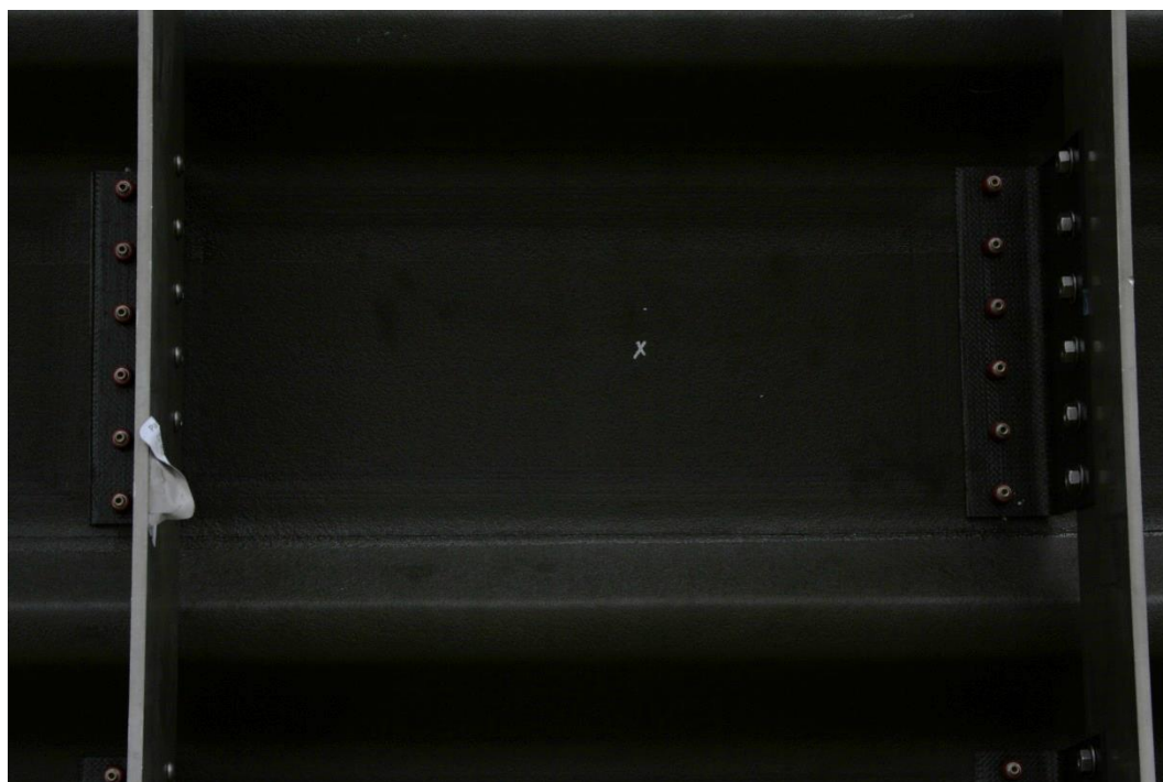
Figure 93. Type I: Back of SP042 (295.4 J).
