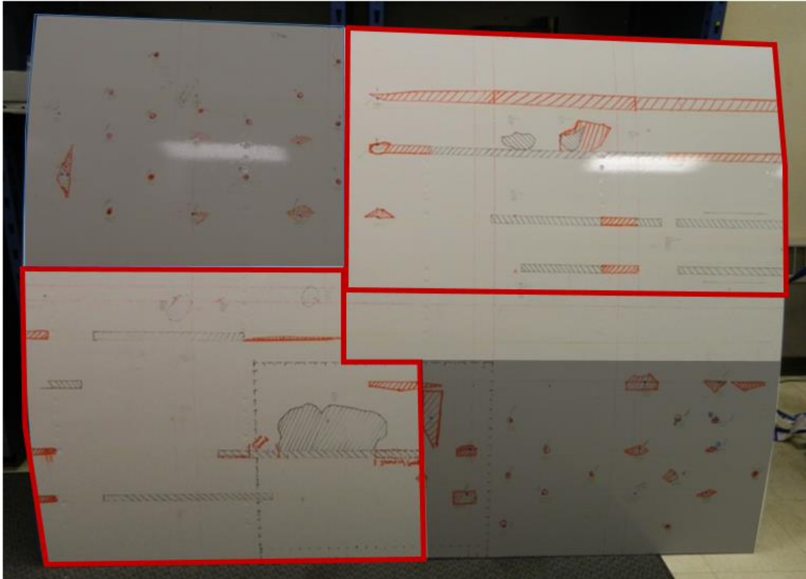
Figure 44. Damage Mapping of Panel A using A-Scan. Black markings show damage detected using NDT Automation CBRZ5X2 SN:282 by UC San Diego. Additional damage detected using MAUS V pulse echo unit by Sandia National Labs is marked in orange. The red boxes emphasize areas impacted by SHI.
