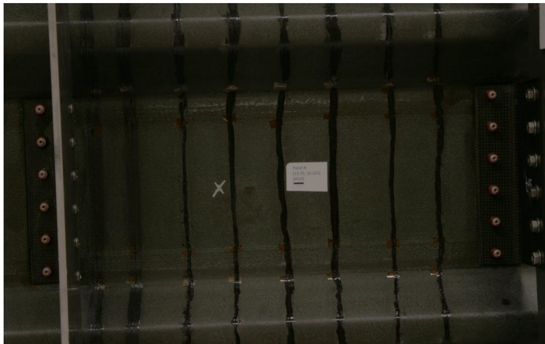
Figure 58. Type I: Back of SP010 (562.3 J).
