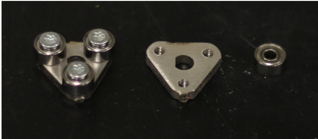
Figure 9.11: Laser cut and tapped sprued stainless steel rotor bodies Note the half-moon driveshaft hole. Laser cutting and tapping operations are performed with multiple sprued parts for ease of handling, then cut out using a rotary tool.
