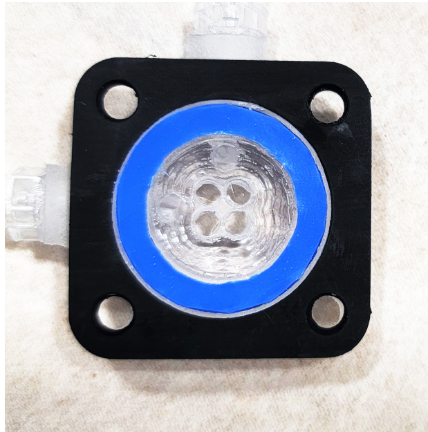
Figure 9.8: Double gasket for organoid cell culture device An inner fluorosilicone gasket is surrounded by an outer isobutylene isoprene rubber gasket.
