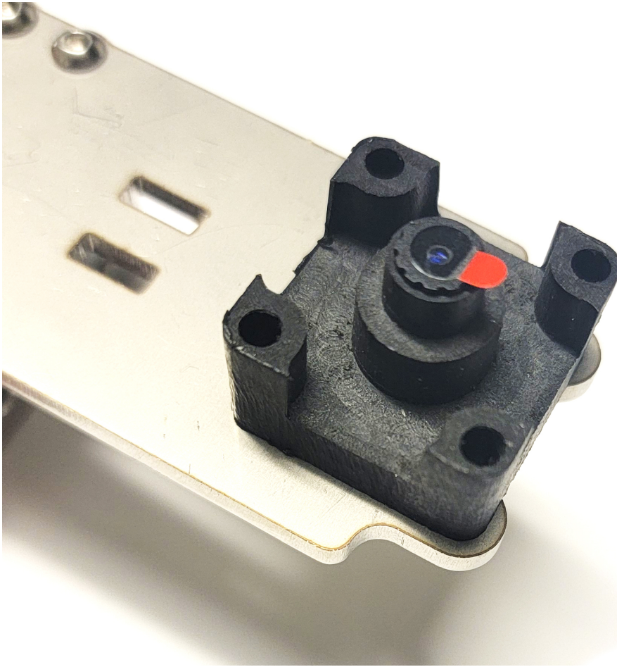
Figure 5.4: Detail of lens extension tube mounted to baseplate A polycarbonate CNC milled extension tube, designed for a single camera device, holds a lens taken from an OV5460 camera module. A friction fit is used to hold the lens. The extension tube shown has four corner posts to hold an LED illumination ring.
