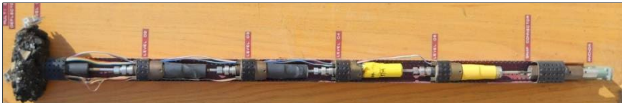
Figure 5.3: A model multi-depth deflectometer (MDD), showing five modules.
