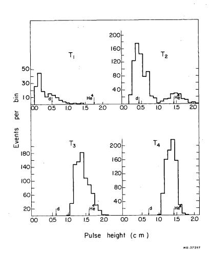
Fig. 16(a). Pulse height spectra determined from oscilloscope film for magnet-system momentum  $P(He^4) = 1060 \text{ MeV/c}$ . Spectrum of T, counter output is based on a scan of only a few events (160): spectra of the other counter outputs are based on a scan of approximately one-third of all the data. Arrows indicate medians of the calibration pulse height spectra for d's and He<sup>4</sup>'s obtained with d and He<sup>4</sup> beams, respectively, from the cyclotron.
