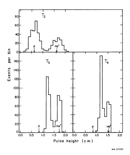
Fig. 17. Pulse height spectra determined from oscilloscope film for magnet-system momentum  $P(\text{He}^4) = 872 \text{ MeV/c}$ . Spectra include approximately one-half of all the data. The pulse heights of the various counters are correlated. Arrows indicate medians of the calibration pulse height for d's and He<sup>4</sup>'s.
