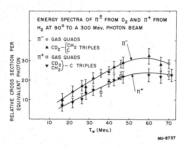
Fig. 4. Energy spectra of  $\pi^{\pm}$  from  $D_2$  and  $\pi^{+}$  from  $H_2$  at 90° to a 300-Mev photon beam.
