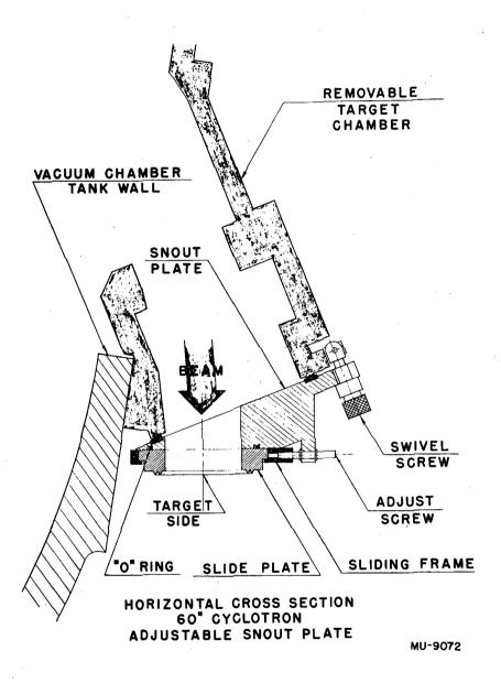
Fig. 2. Horizontal cross section, 60-inch cyclotron, adjustable snout plate.
