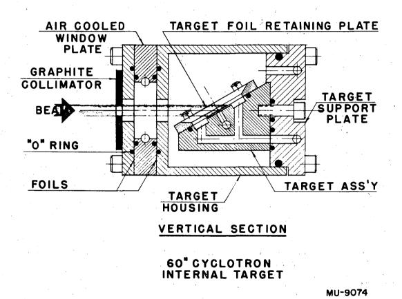
Fig. 4. Sixty-inch cyclotron, internal target, vertical section.
