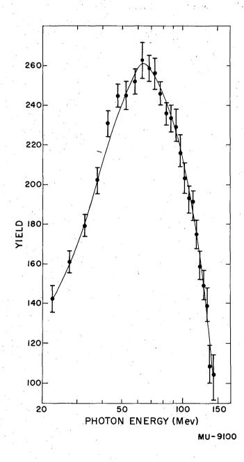
Fig. 1. Total spectrum from 340-Mev proton bombardment of carbon.
