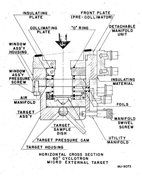
Fig. 3. Horizontal cross section, 60-inch cyclotron, external microtarget.
