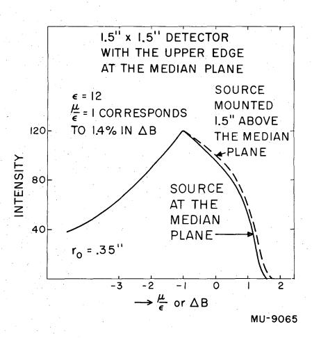
Fig. 6. Effect of Z focusing on resolution curve with  $\sim 15^{\circ}$  slit near detector.
