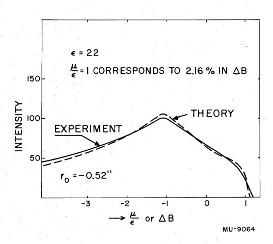
Fig. 5. Resolution curve with no slit near detector.
