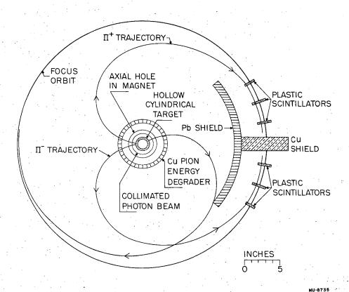
Fig. 2. Experimental arrangement for photomeson production.
