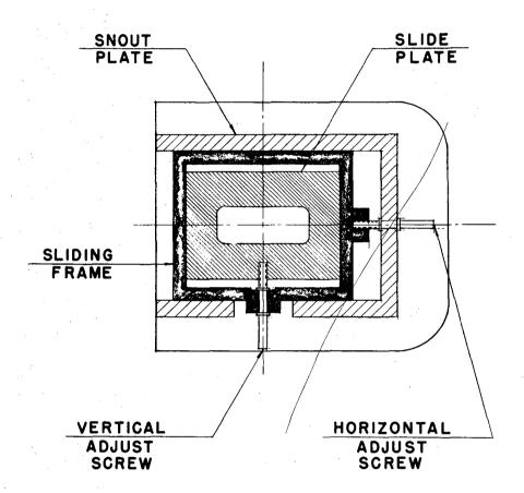
SCHEMATIC LAYOUT 60" CYCLOTRON SNOUT PLATE 2 WAY ADJUSTMENT
