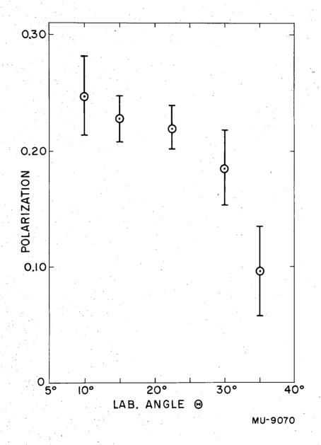
Fig. 7. Polarization P versus laboratory-system scattering angle (H) for proton-proton scattering at 170 Mev.
