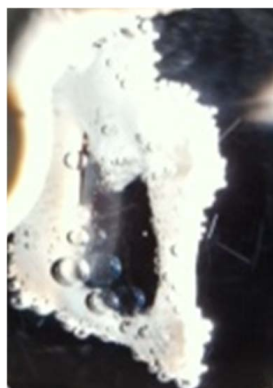
Figure 3-21: Bubbles generated at the surface of the NiO x |Ni|InGaN/GaN MQW photoanode.
