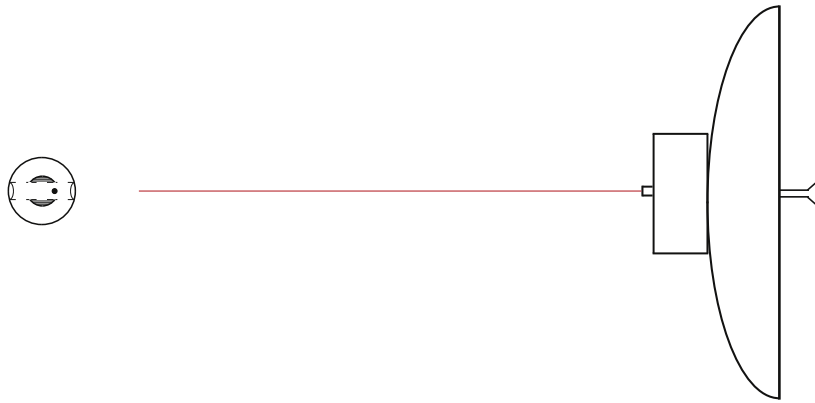
Figure 1. Schematic of our proposed experimental setup. The smaller retroreflector exhibiting harmonic motion within the tunnel of the larger mass is represented by the black circle (on the left). Determinations of the round trip light-time from the host spacecraft (on the right) to the retroreflector using an onboard ranging system provide measurements of the period of the gravity train oscillator.
