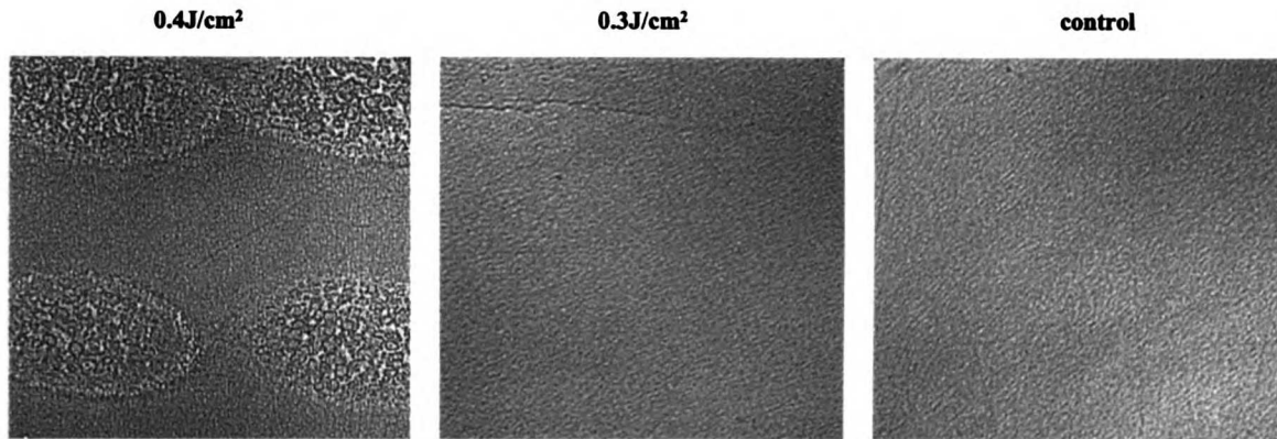
Figure 6. Bovine enamel surfaces after irradiation with 9.6 \mu\text{m} laser beam at the fluences shown, and untreated control (magnification 500x).
