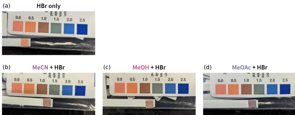
Figure S10. pH of (a) concentrated hydrobromic acid or mixtures of (b) acetonitrile, (c) methanol, and (d) methyl acetate with HBr in a 3:1 ratio.
