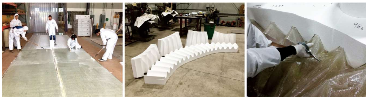
Figure 18. The sandwich core is made from a thin layer of glass-fiber reinforced plastic (GFRP) and pressed into form using a Styrofoam mold that was custom-made on a 4-axis hotwire machine.
