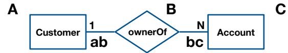
Figure 1: Geometric configuration of an ER diagram. Labels '1' and 'N' denote that one customer may have many accounts, but a single account belongs to one customer. The remaining letters label the closed curves and the lines.
