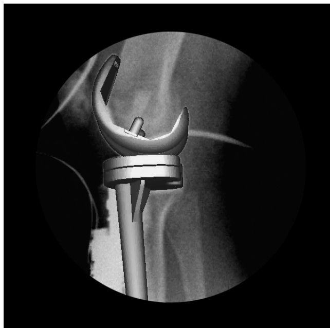
Figure 18B: The processed fluoroscopic image has been overlaid with the CAD models oriented at the shaped matched site.
