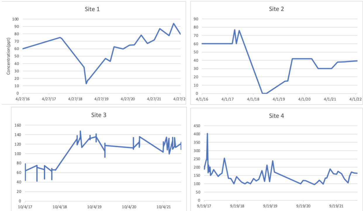
Figure 3.1 Fluctuations in total PFAS yearly concentrations of four sites. The vertical axis represents the total PFAS concentration, and the horizontal axis shows the sampling dates; the unit of the PFAS concentration is part per trillion (ppt). The PFAS subclasses amount tested, and species considered are the same within the four sites.
