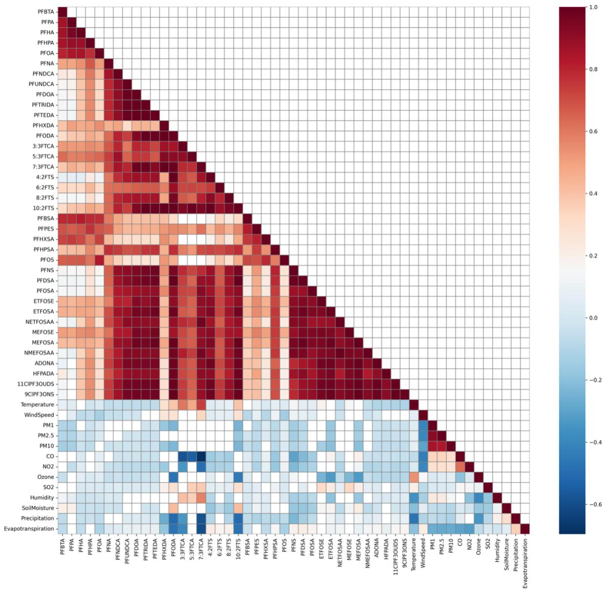
Figure 3.8. The Spearman's rank ( $p < 0.05$ ) correlation coefficient heatmap plot for PFAS and soil, air, and weather factors. The red color indicates a positive correlation, and the blue color represents the negative correlation between each of the two parameters, the darker the relationship between them is more robust.
