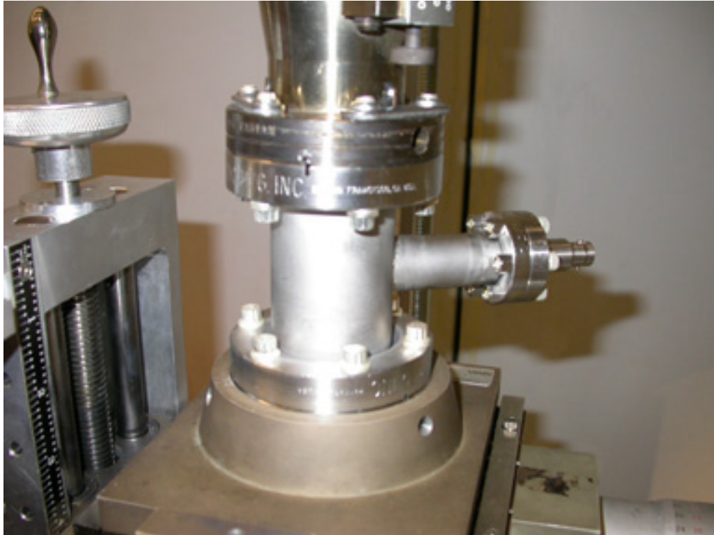
Figure 5.46. Electrical feedthrough for tunneling current signal is located away from the rest of the electrical feedthroughs for shielding of the output.
