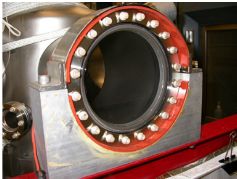
Figure 5.53. The system is secured onto the carbon steel framed through a series of silicone-lined ring clamps, each mounted onto a flange on the transfer arm axis.
