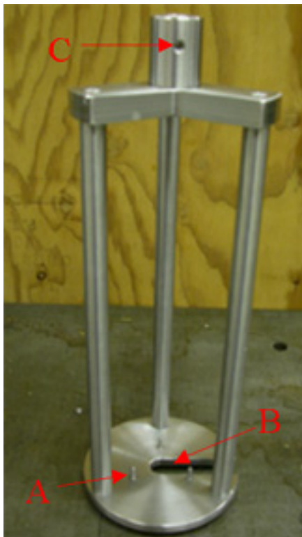
Figure 5.41. The docking scaffold (before incorporation of storage stations) contains three chamfered pins ( A ) to be mated with the corresponding holes under the pressure cell. A rectangular notch ( B ) allows routing of gas from the lower connection of the pressure cell. The scaffold can be mounted onto a XYZ \ominus manipulator by two 4-40 set screws ( C ).
