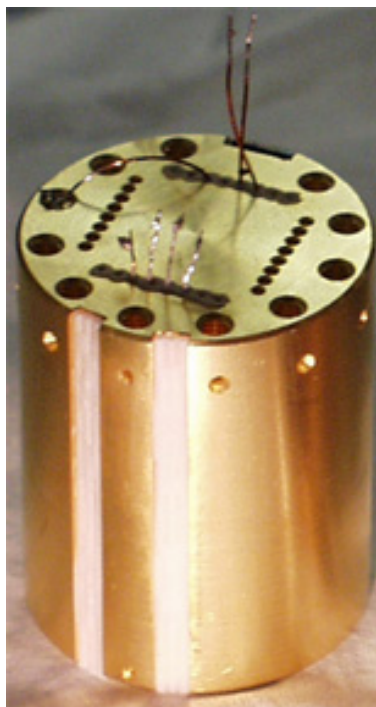
Figure 5.7. Rear view of the STM body, now gold-plated, shows the alumina tubing inside the back trenches, before the trenches are electrically shielded with a covering gold foil.
