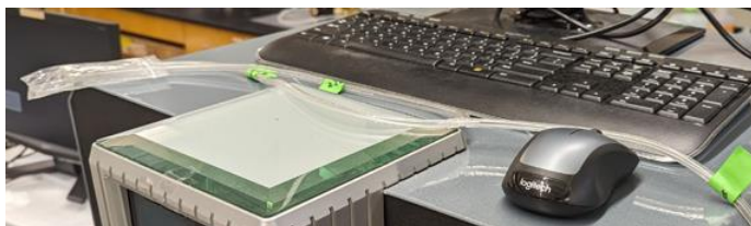
Figure GA.4.12. Laser split Teflon tube prior to connection to ICP. Both the glass flange and carrier gas end are in the plastic bag.
