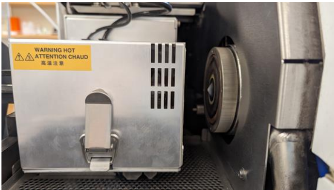
Figure GA.4.8. Inside of ICP housing with sampler cone visible. Skimmer cone inside/behind the sampler cone (not visible).
