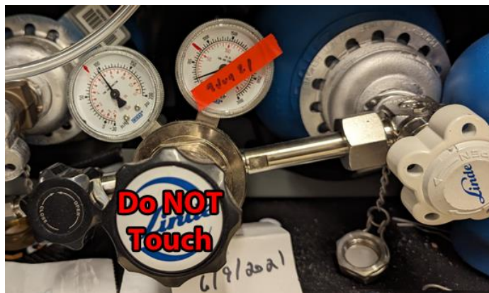
Figure GA.4.3. Picture of ArF tank valves. White valve on the right opens/closes the ArF tank. Middle valve labeled, “Do NOT Touch,” sets the pressure leaving the tank (pressure regulating valve). Black valve on the left opens/closes the path to the laser cell. Pressure in the tank is measured on the right gauge with tape over the starting pressure and red mark on the time to order a new tank pressure. The pressure regulating valve is set to be the pressure of the red mark.
