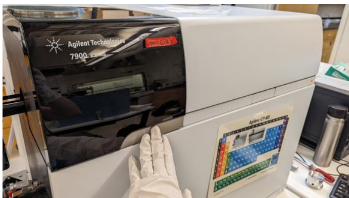
Figure GA.4.7. ICP with gloved hand on the silver button of the housing box. Red tape on the top left of the housing box denotes which sampler and skimmer are currently in the ICP.
