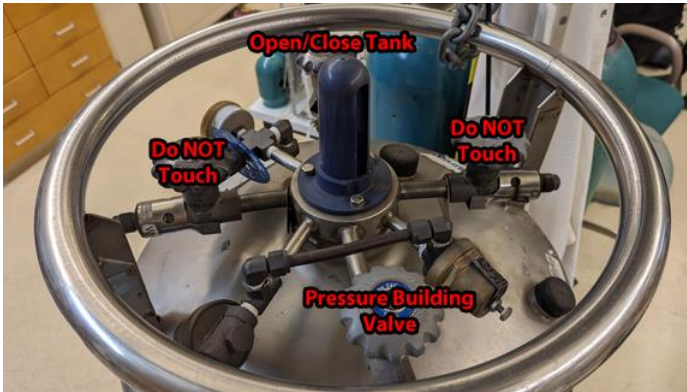
Figure GA.4.16. Labeled valves on liquid Ar tank.
