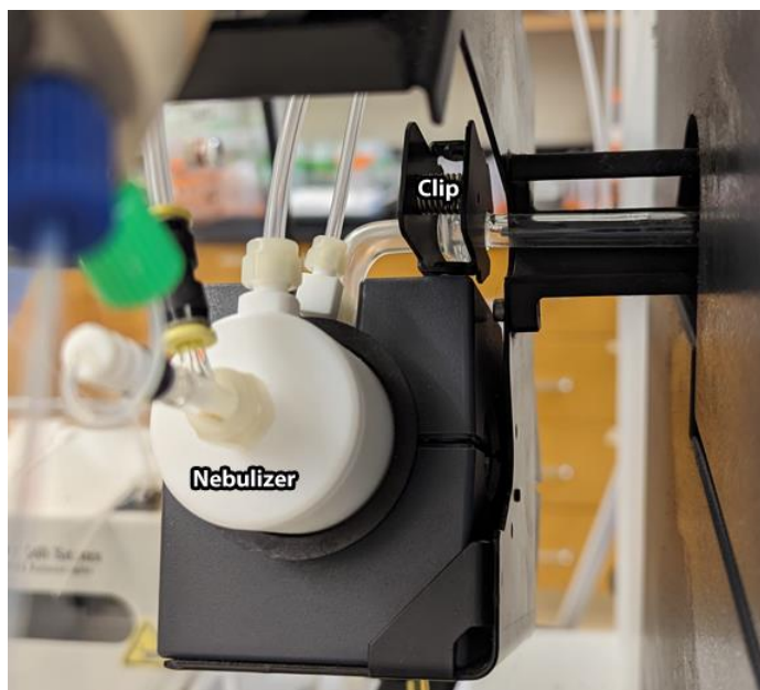
Figure GA.4.11. Picture of the Nebulizer and clip attaching the nebulizer to the ICP. Screw under the nebulizer is not in view.
