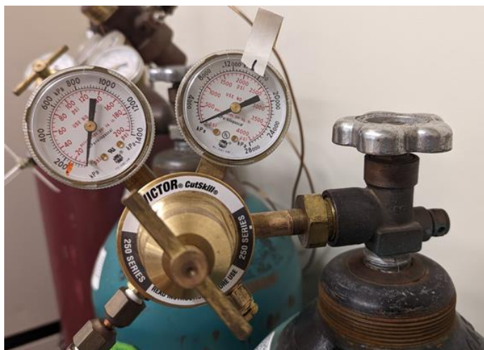
Figure GA.4.1. Picture of N_2 tank valves. To open the N_2 valve, rotate the left, silver-colored valve counter-clockwise. Do not touch the pressure regulator valve, the brass valve beneath the gauges. Gauge on the left is the pressure regulator gauge that displays the pressure of the gas leaving the tank. Orange mark denotes where the pressure regulator should be set. The gauge on the right is the tank pressure gauge which shows how much gas is in the tank based on the gas pressure in the tank. White tape with black line marks the tank starting pressure.
