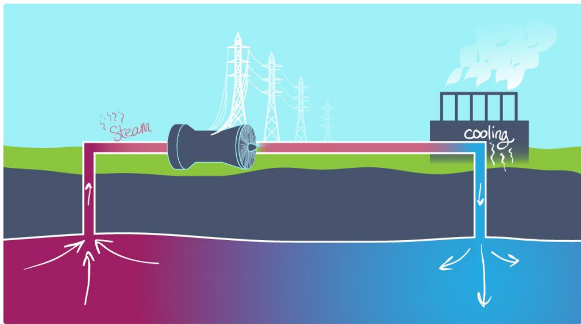
Figure GA.2.6. Scientific illustration of geothermal energy production. Energy is produced in this system by extracting hot, geothermal brines and allowing them to cool to a point that steam is generated. The steam moves a turbine which generates electricity. The brine is further cooled before it is reinjected back into the geothermal reservoir where it heats back up and is re-extracted.
