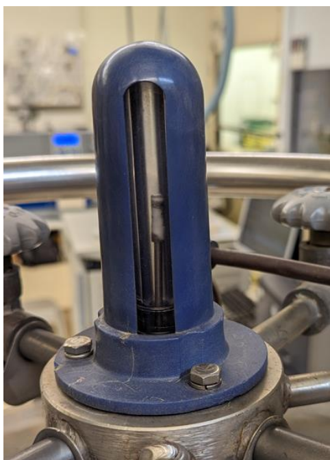
Figure GA.4.4. Picture of Ar tank liquid volume gauge. There are multiple different types of gauges that could be used but they are not the most accurate and sometimes fully broken. This gauge is always located at the top of the liquid Ar tank (first tank you will see when you enter the lab space from the hallway).
