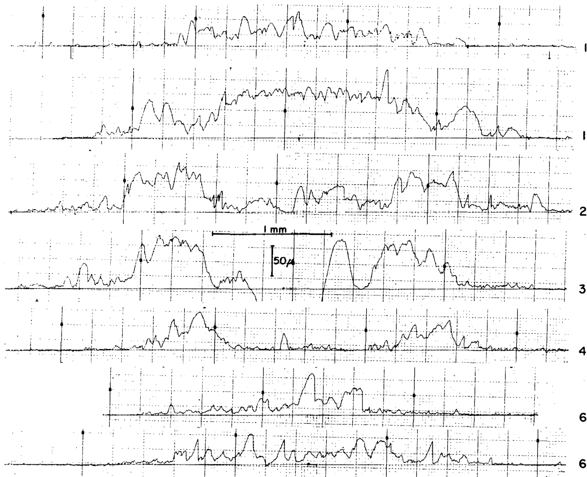
Fig. 15. Profiles made normal to the centerline of the wake around a nonconducting sphere. The respective positions of each profile is given in Fig. 13.
