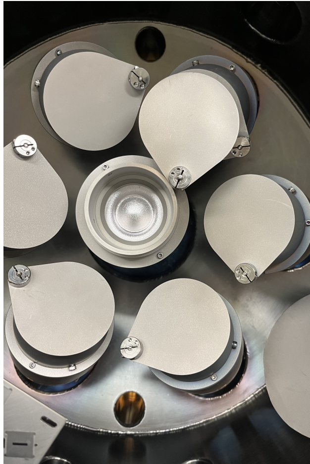
Figure 3.2: Seven sputtering guns on the ATC-2000F deposition system are shown housed in chimneys. Chimney shutters are swung open when making a deposition. As targets reach the end of their lifetime, deep circular rings become prominent on their surface.
