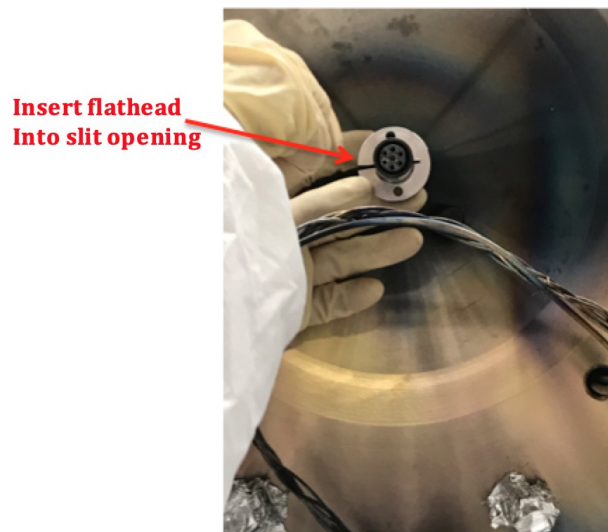
Figure A.47: Remaining support clamp after the reflector box has been removed from the pole piece
