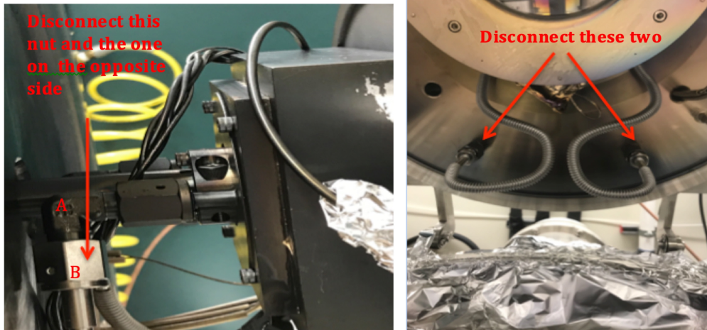
Figure A.34: Left: Disconnect nut B and the identical one on the opposite side (unpictured). Right: Disconnect these VCR connections at the points shown
