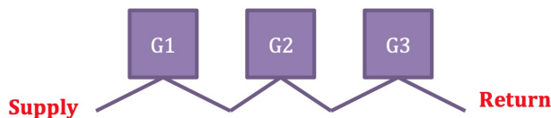
Figure A.24: Example of how water lines for guns are connected in series
