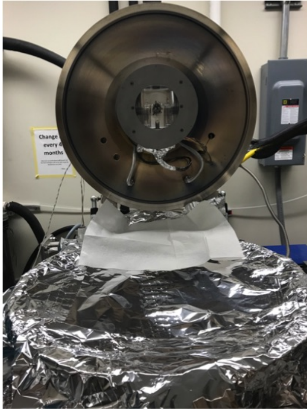
Figure A.37: Ensure the chamber opening is covered and protected before checking for water leaks
