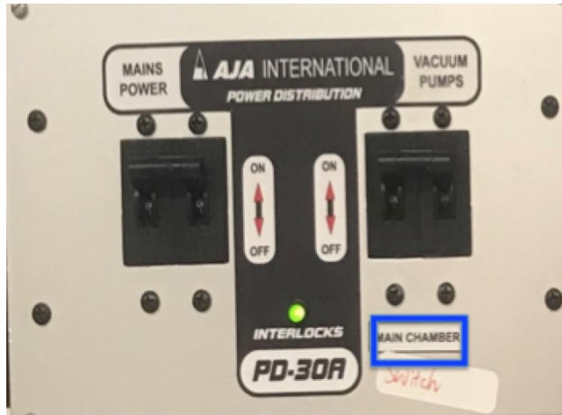
Figure A.15: Controller for main chamber vacuum pumps and their power– turn vacuum pump off to stop the turbo pump
