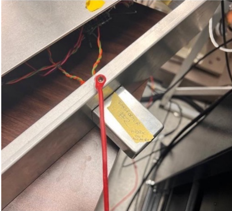
Figure 3.47: A 1:1 audio transformer is soldered to the back of the Wheatstone bridge. This is a crucial component which seems to be removed from the several spare bridges currently in lab storage!
