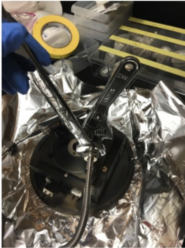
Figure A.35: Example of how to disconnect connections pictured in Fig. A.34—hold nut A fixed with one wrench and rotate nut B with a second
