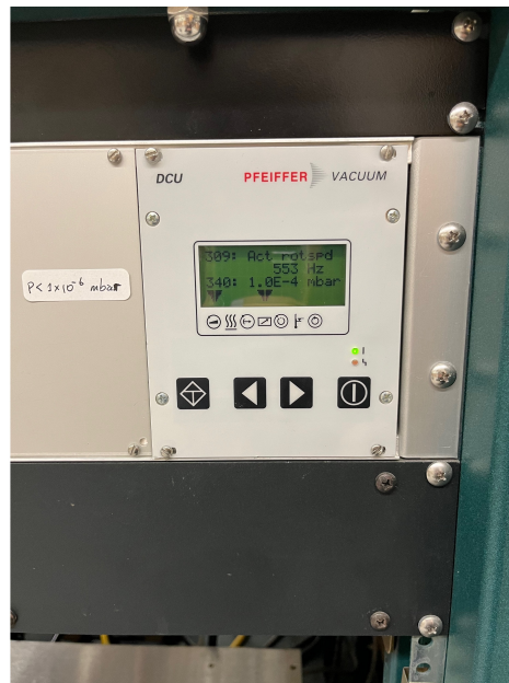
Figure A.6: Use scroll keys 4 and 5 on the load-lock DCU display to read turbo pump power, current, and rotational frequency.
