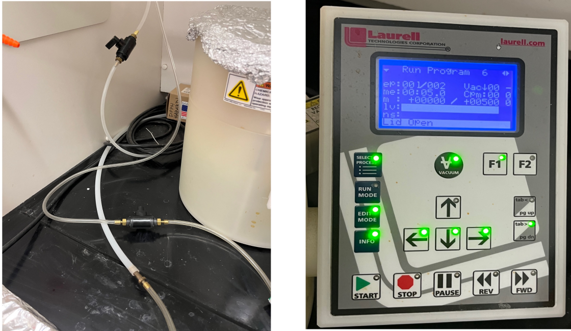
Figure 3.25: Black valves for controlling vacuum level (left) and keypad controls (right).
