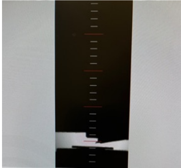
Figure 3.11: Silhouette of the AFM tip while being lowered to the sample surface using the Head Stage controls. Lower the tip to within one notch mark of the sample surface.
