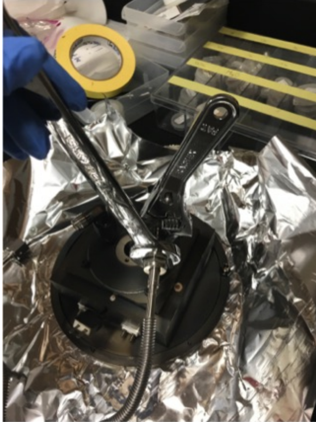
Figure A.49: Hold elbow tee fixed with one wrench and rotate the female nut with another
