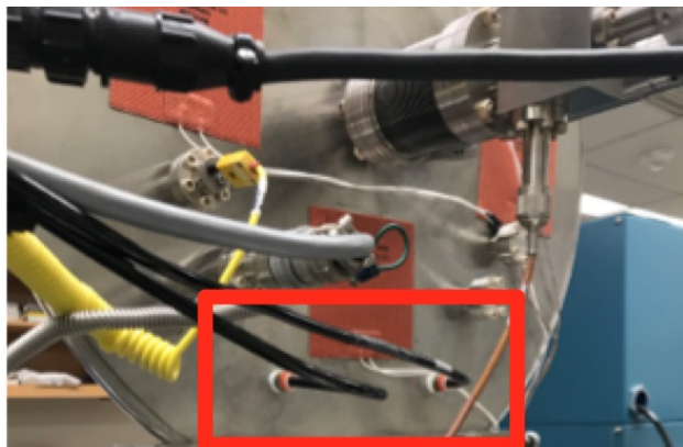
Figure A.38: Keep the chamber lid vertical and re-insert the water lines back in as normal
