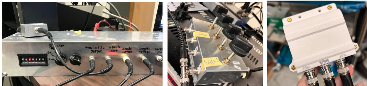
Figure 3.48: Components of the AMR setup: grounded Wheatstone bridge (left), switchbox (middle), and adapter (right).
