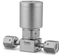
316L VIM-VAR UHP Diaphragm Sealed Valve, 1/4 in. Female VCR Fitting, SC-01 Cleaned, NC Actuator
