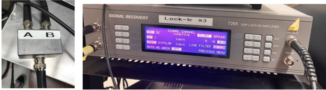
Figure 3.46: A-B splitter (left) and lock-in measurement settings (right). User beware that this Signal Recovery lock-in has problems above 30 dB gain– replace with SRS 380 or use with caution.
