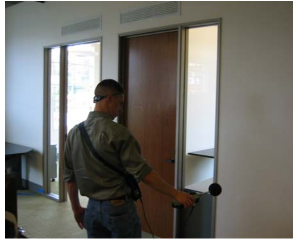
Figure 17. Sound Leak Assessment
