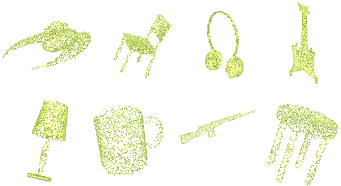
Figure 2.9: 8 3D CAD shape examples from each category of Dataset 6 [1]. From left to right, top to bottom: airplane, chair, earphone, guitar, lamp, mug, rifle, and table.
