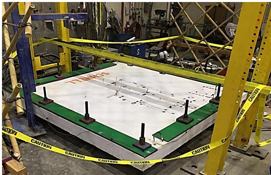
(b) Slab Specimen “B” Test Setup
