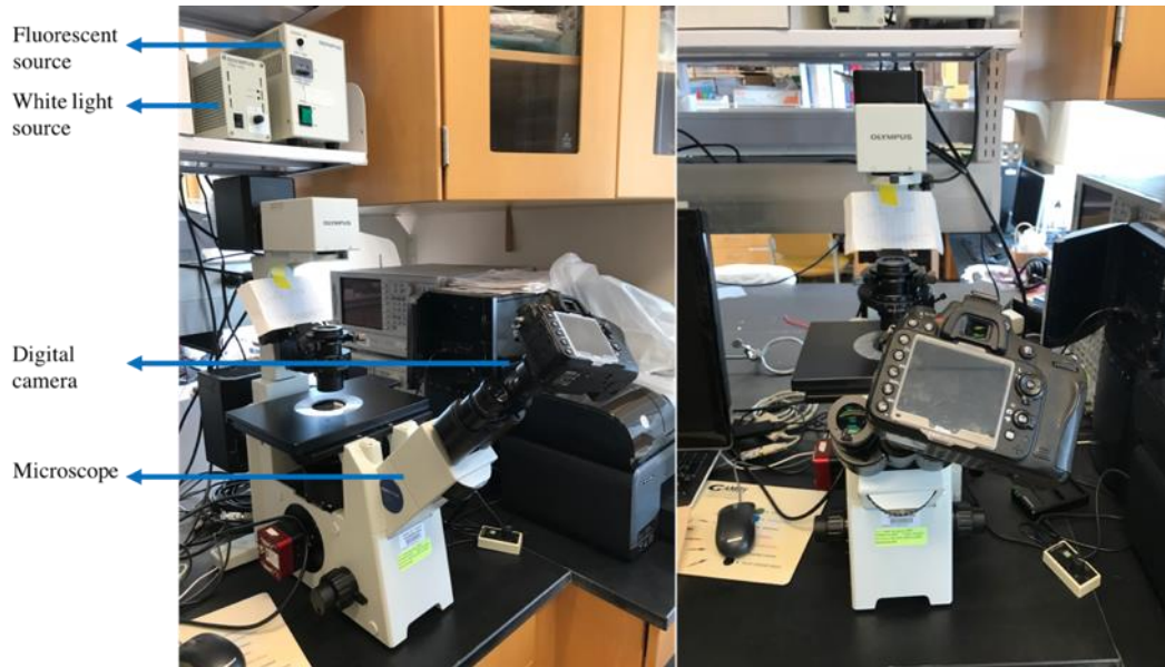
Figure 4-4. Image of inverted microscope used in this study.
