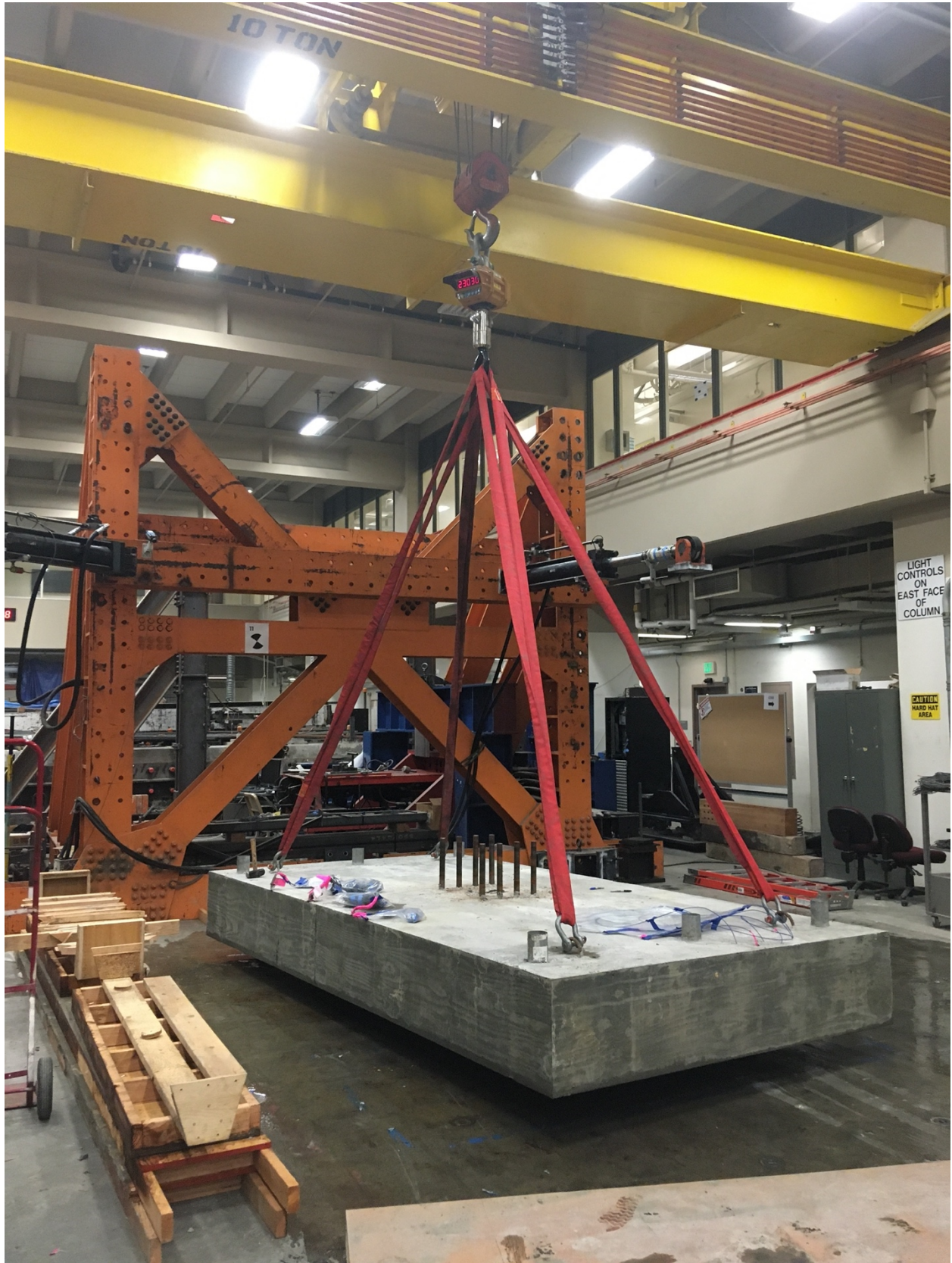
Figure F- 55. Moving specimen with crane
