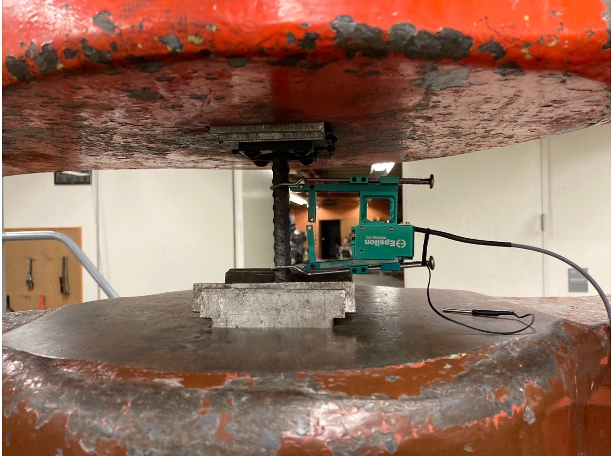
Figure F- 83. Testing shear reinforcing bars with 2" gage extensometer
