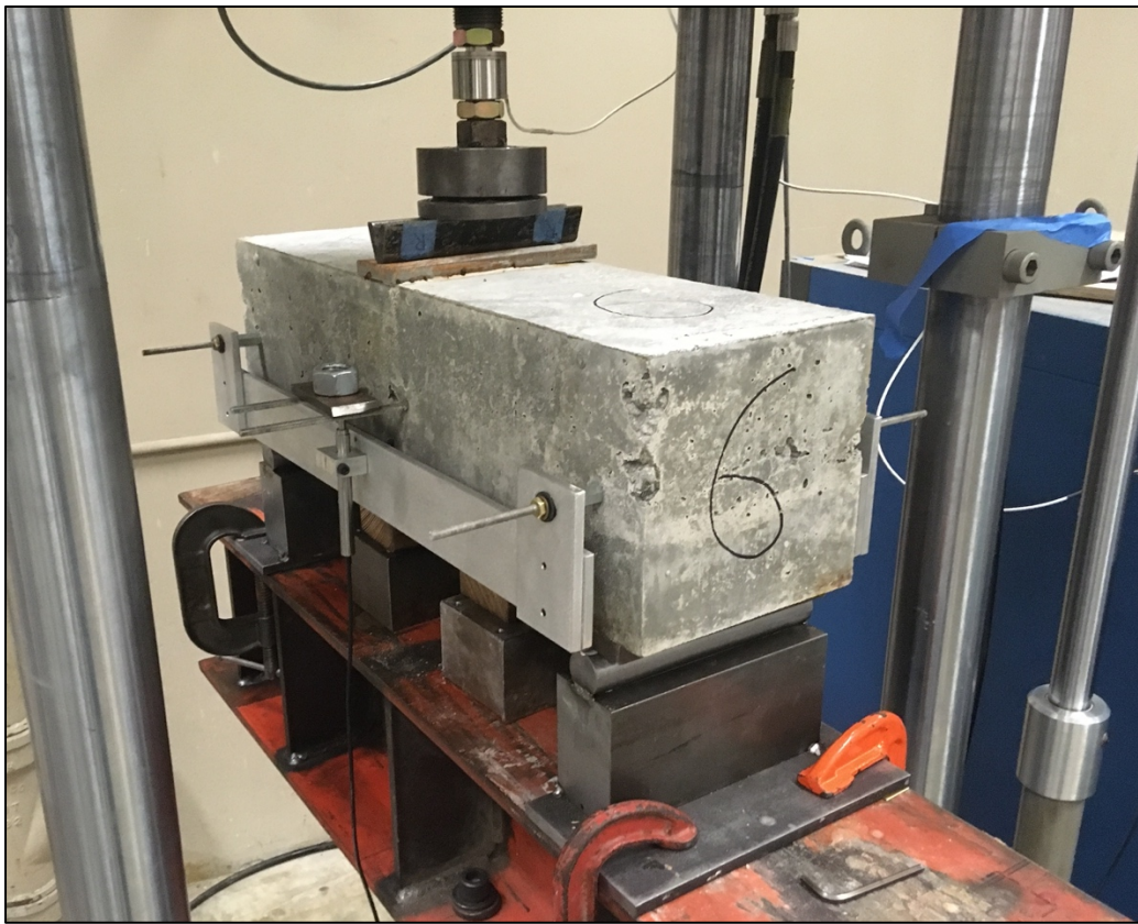
Figure A- 3. Concrete Fracture Energy test set-up
