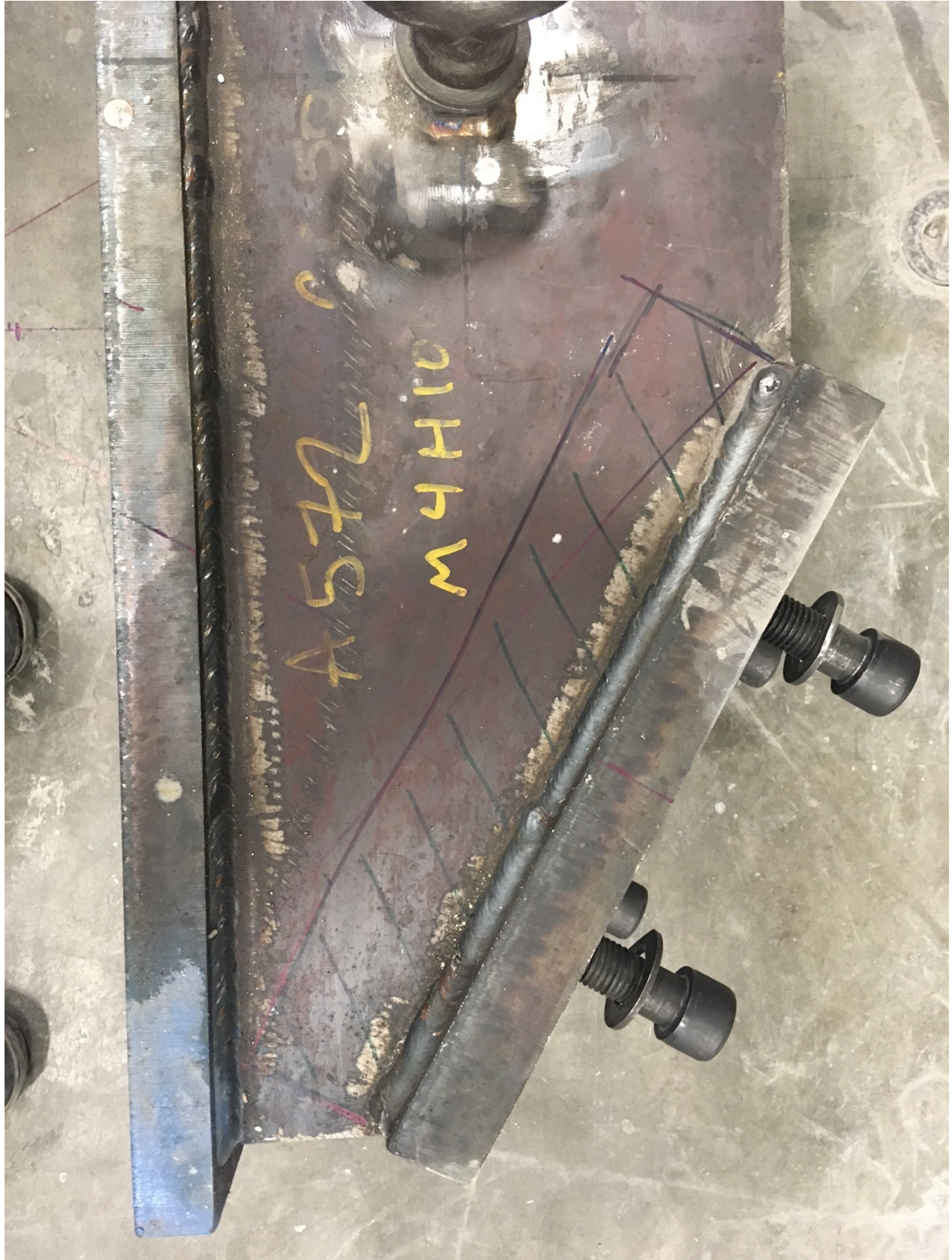
Figure F- 66. Modification to column-actuator attachment
