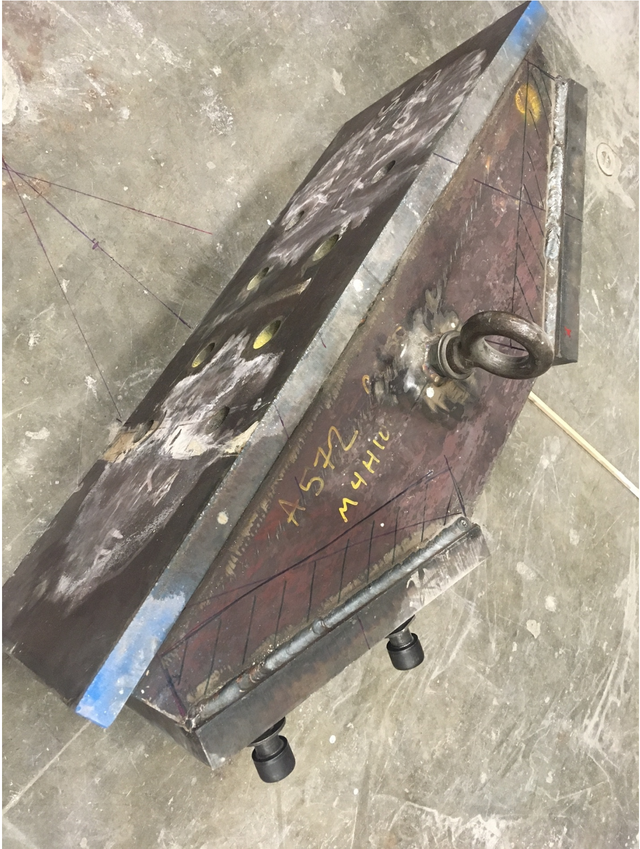
Figure F- 65. Modification to column-actuator attachment
