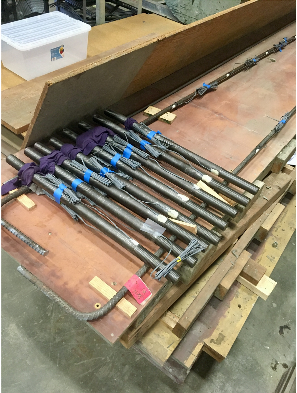
Figure F- 2. Strain gages on anchors
