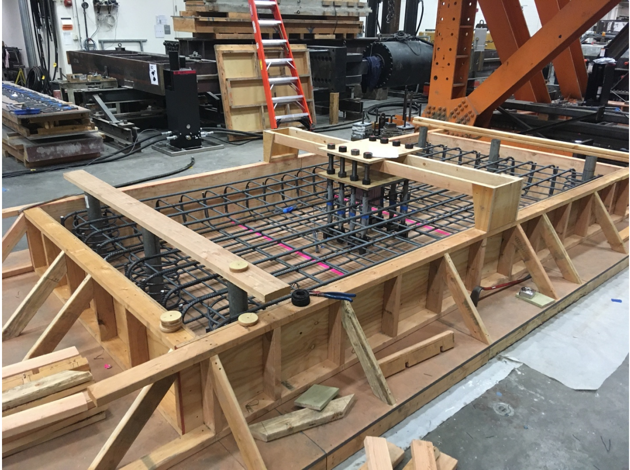
Figure F- 12. Cage building and anchor fixture
