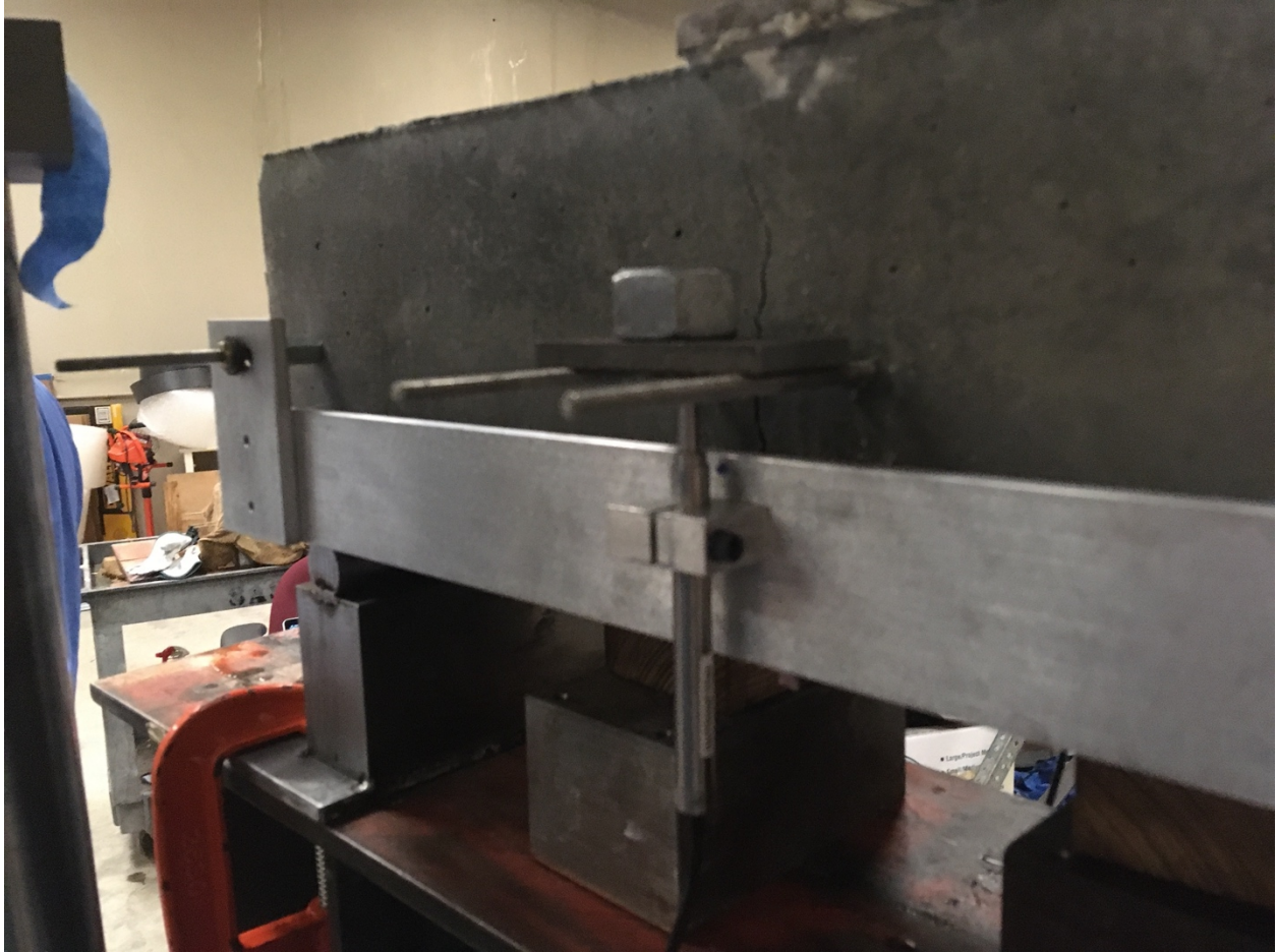
Figure F- 86. Fracture energy tests
