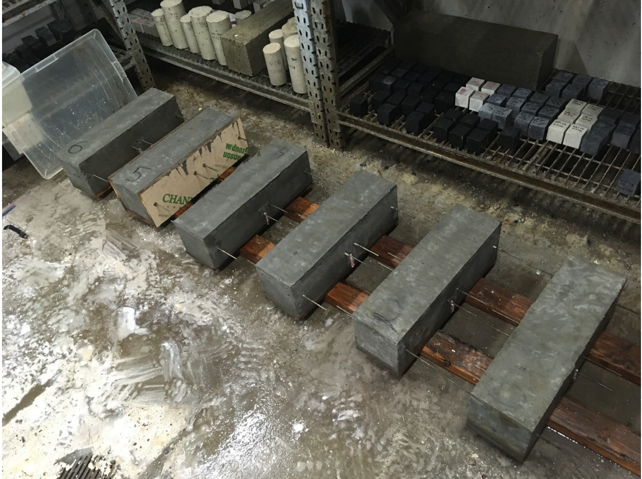
Figure F- 51. Fracture energy beams in fog room
