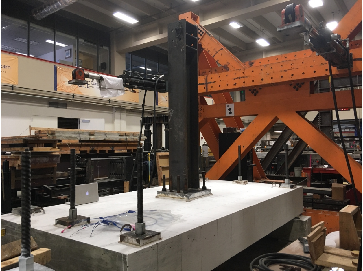
Figure F- 61. Column hydrostoned to specimen
