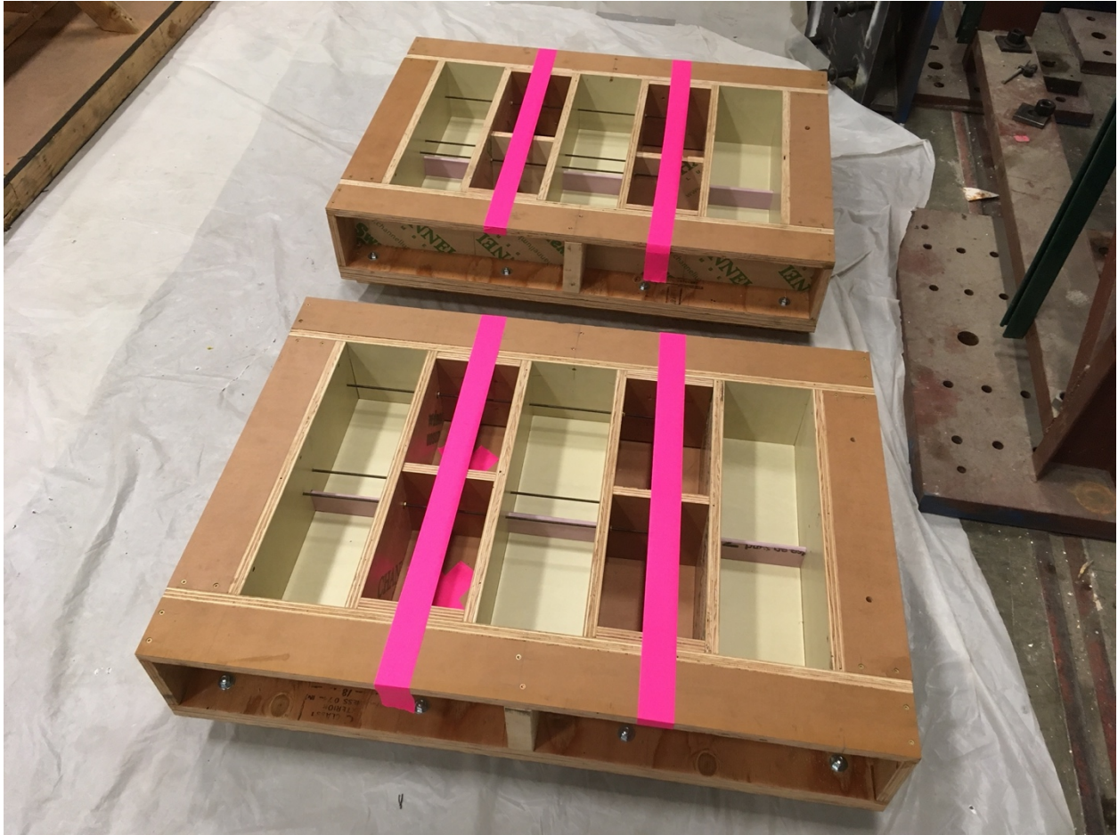
Figure F- 19. Fracture energy forms before casting concrete
