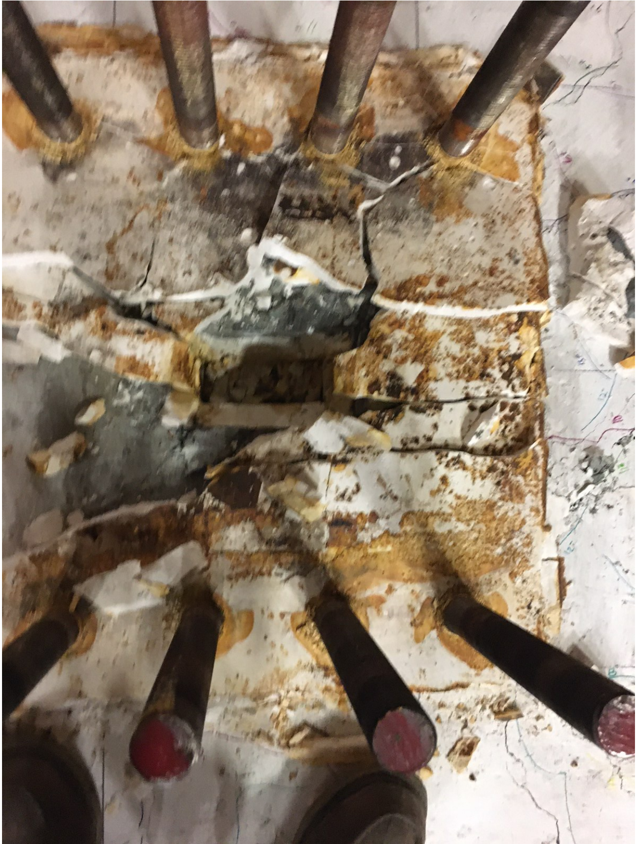
Figure F- 75. Slab plan view after removing column
