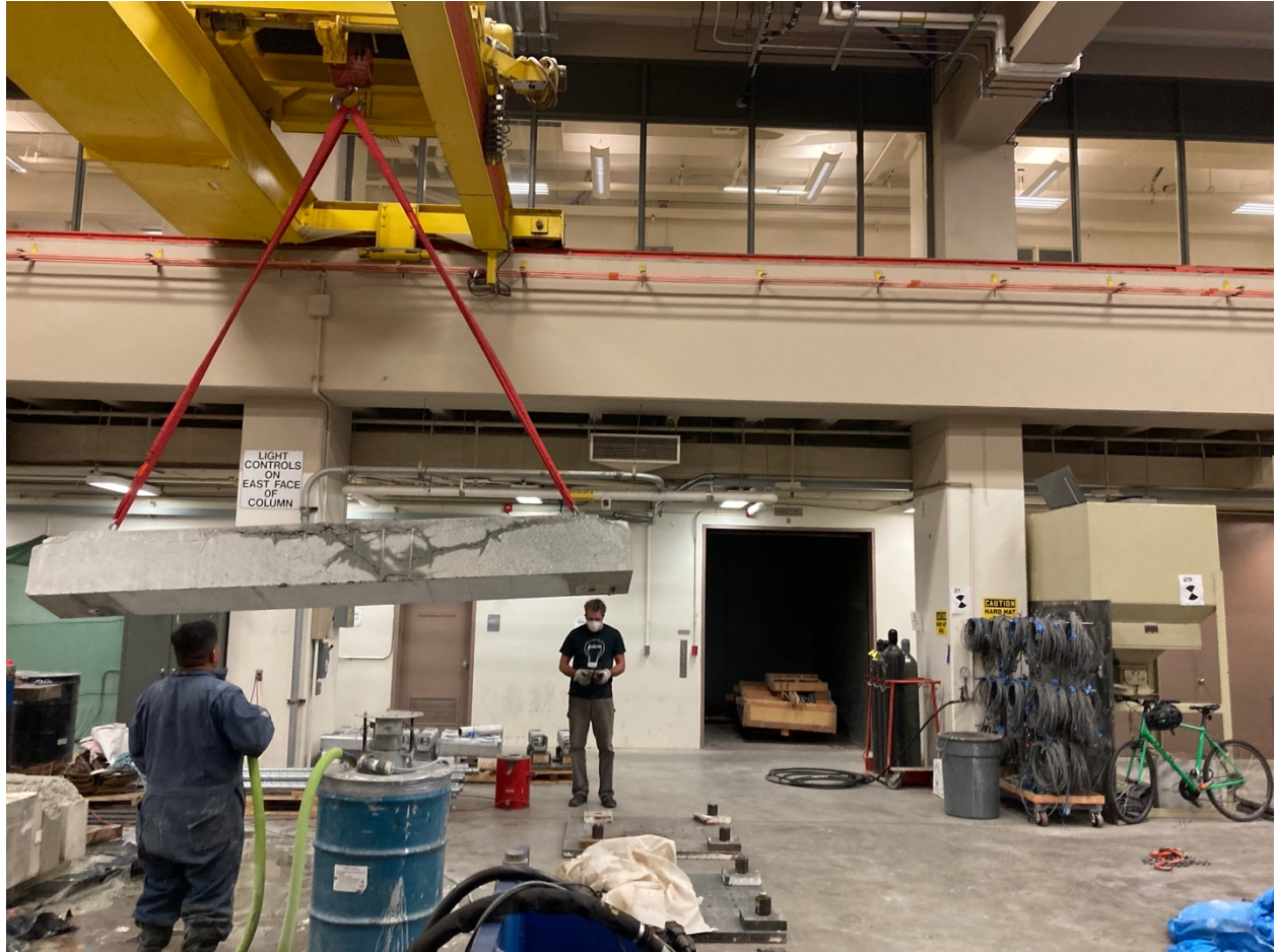
Figure F- 81. Cutting cross sections
