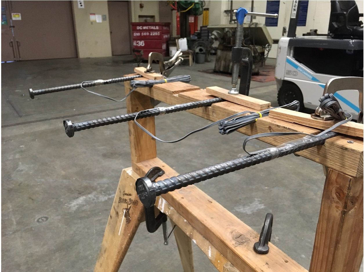
Figure F- 6. Strain gages on shear reinforcement
