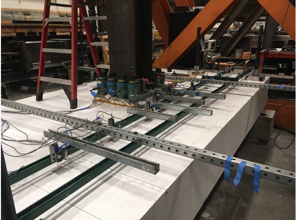
Figure F- 69. Instrumentation frame to attach linear potentiometers to measure vertical displacements
