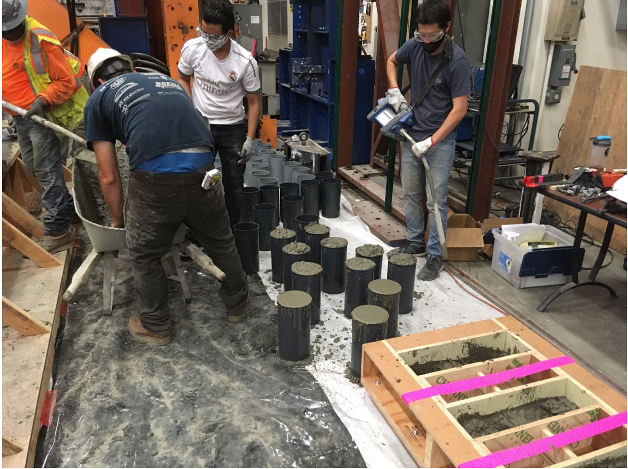
Figure F- 37. Casting concrete
