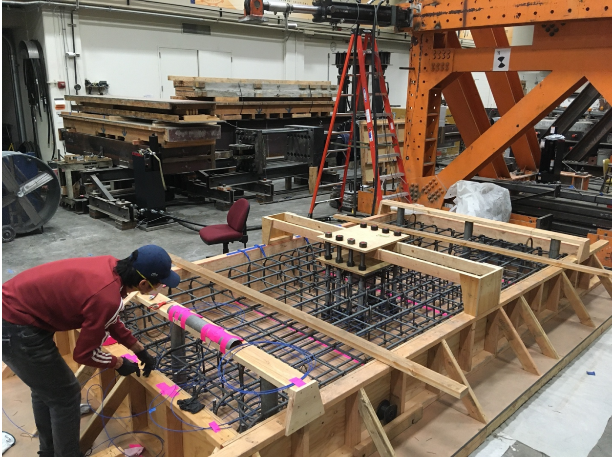
Figure F- 15. Placement of fiber optics cables
