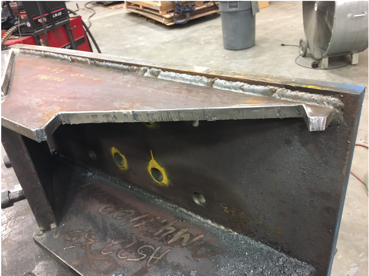
Figure F- 67. Modification to column-actuator attachment
