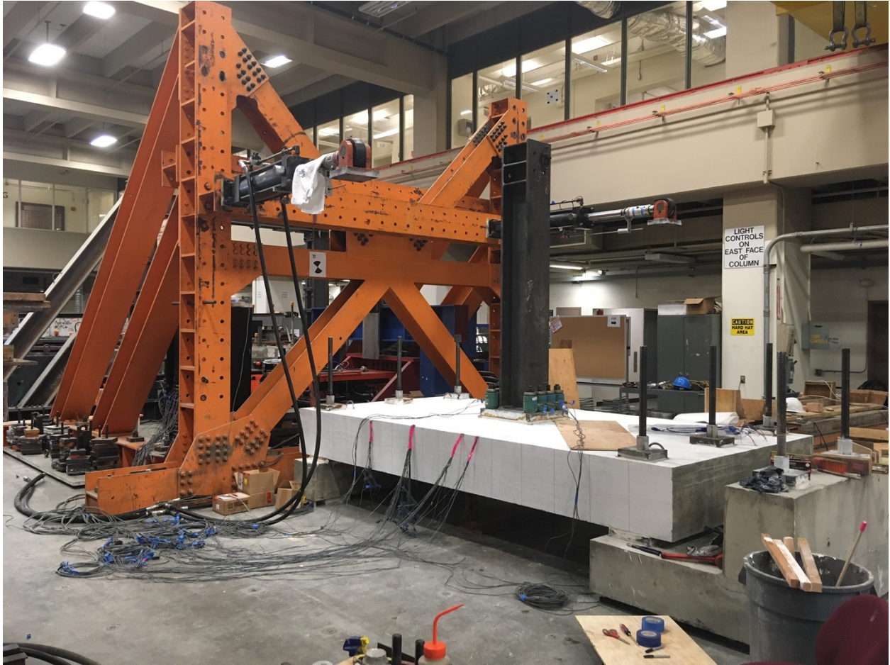
Figure F- 63. Column hydrostoned to specimen and anchor load cells in place
