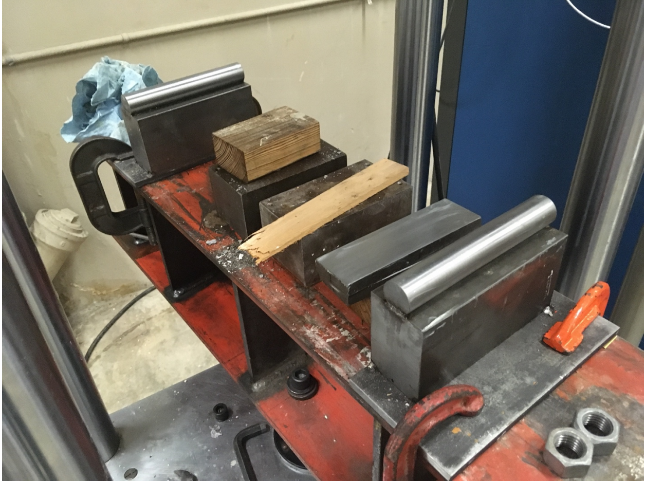
Figure F- 92. Fracture energy tests
