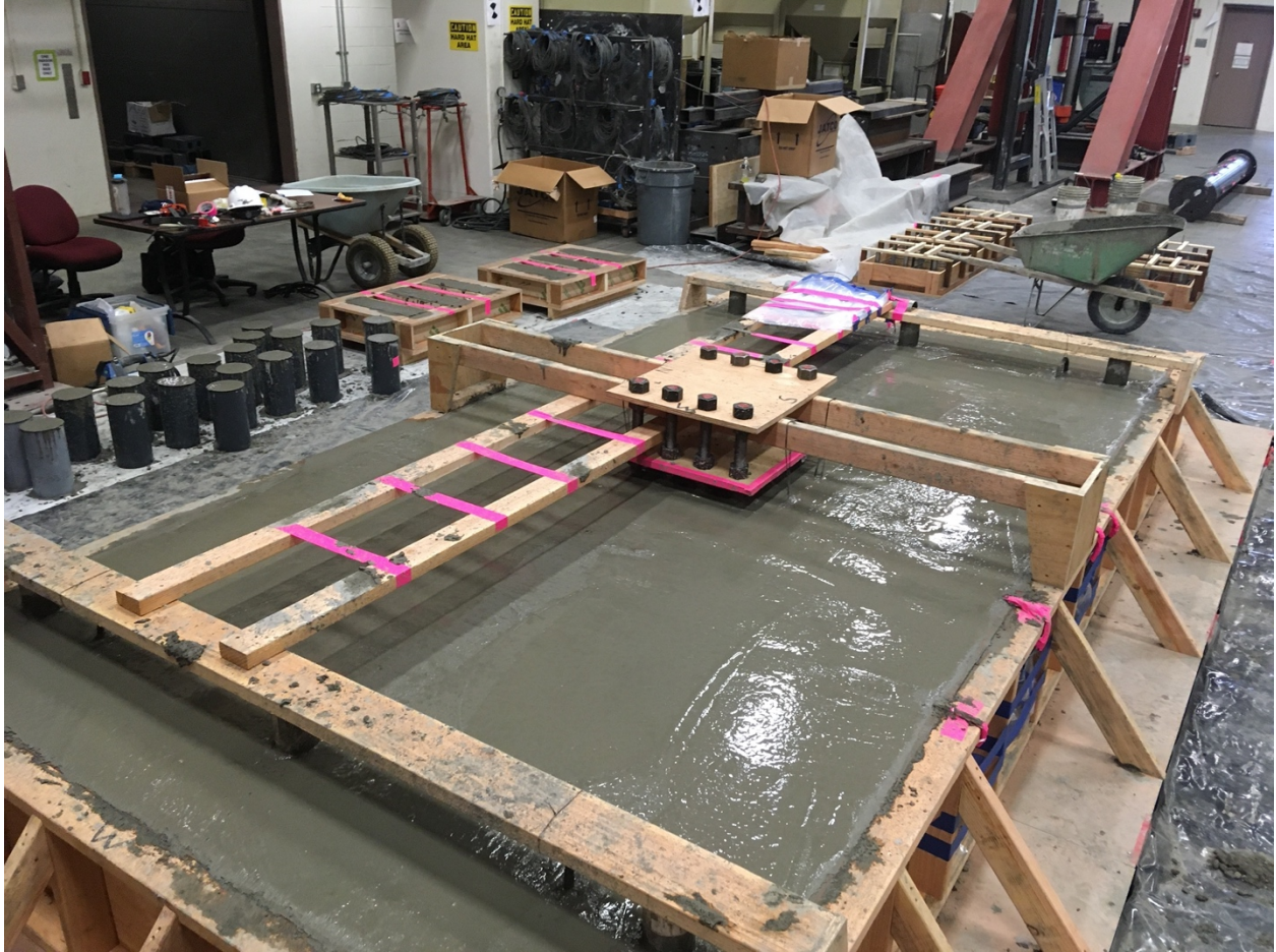
Figure F- 46. Casting concrete
