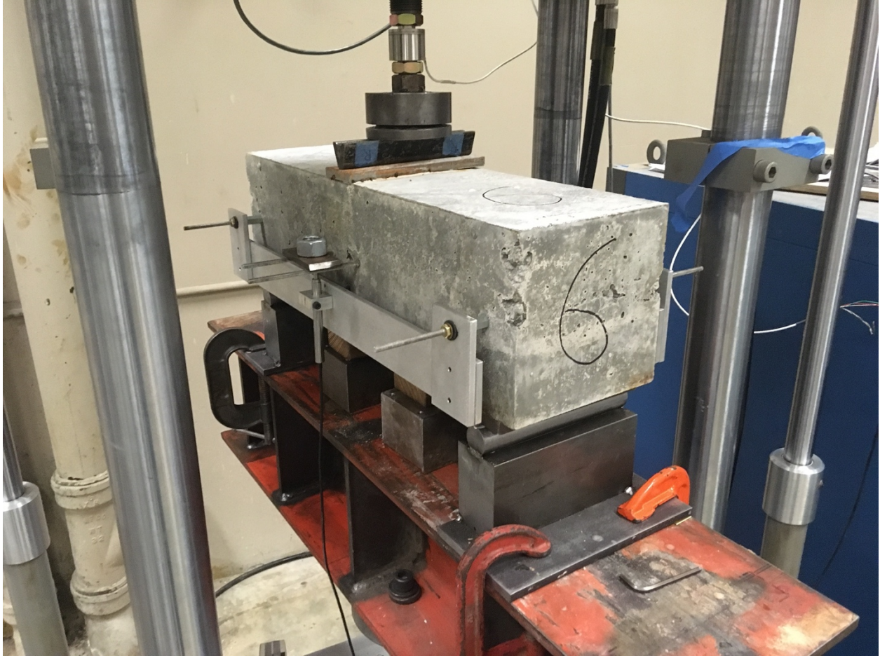
Figure F- 90. Fracture energy tests
