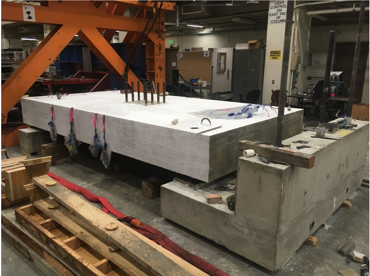
Figure F- 57. Specimen placed on concrete supports
