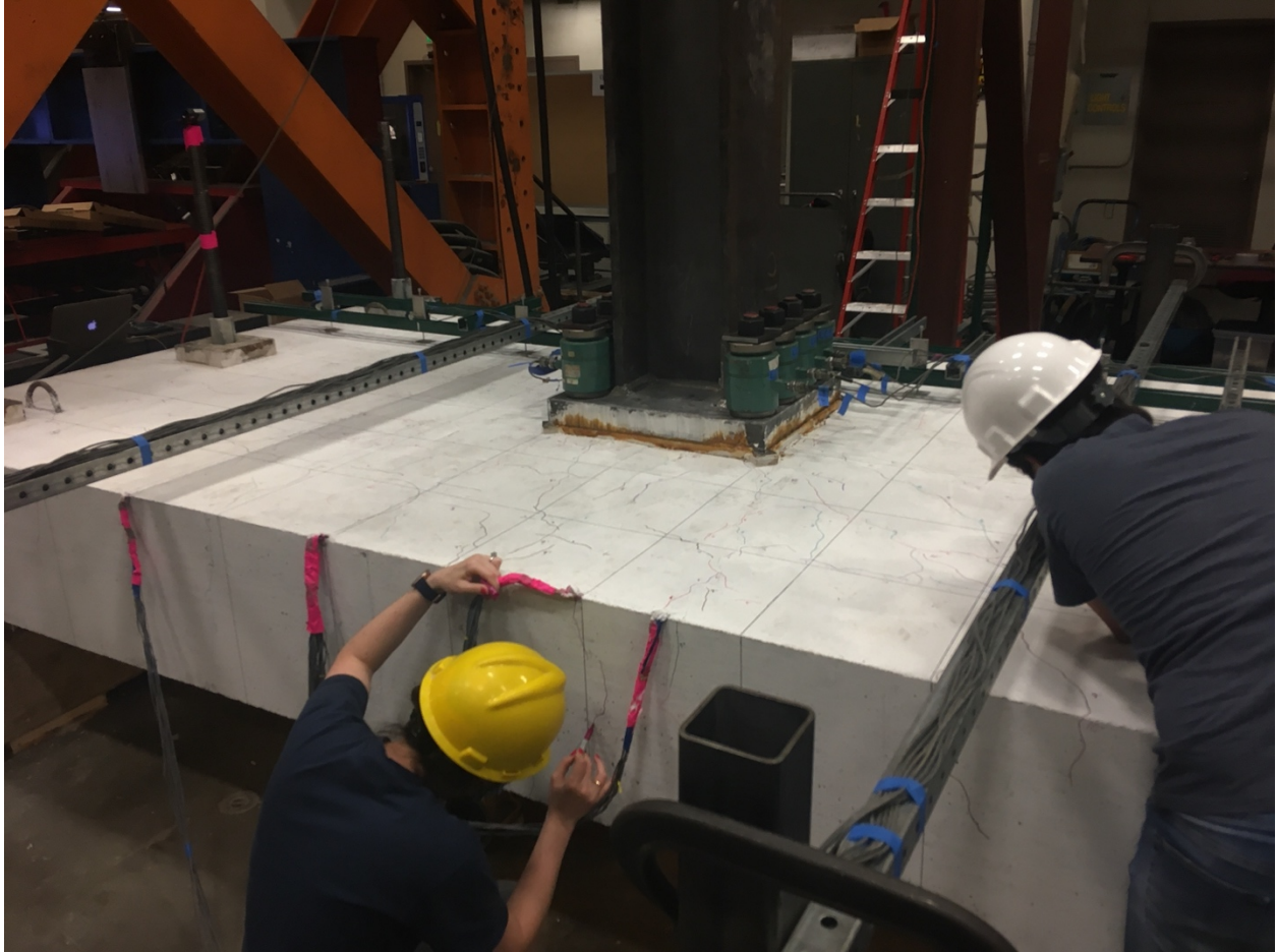
Figure F- 74. Documenting cracks during test
