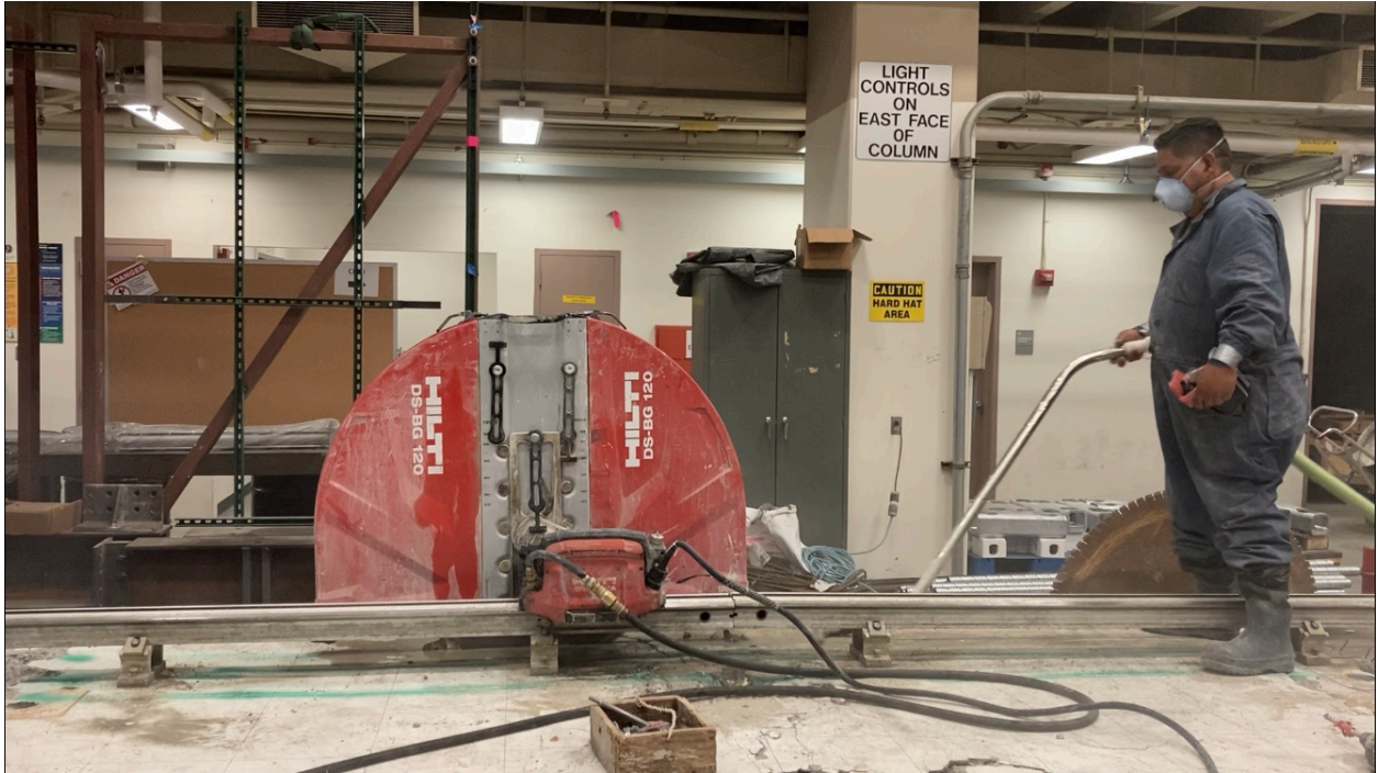
Figure F- 77. Cutting cross sections
