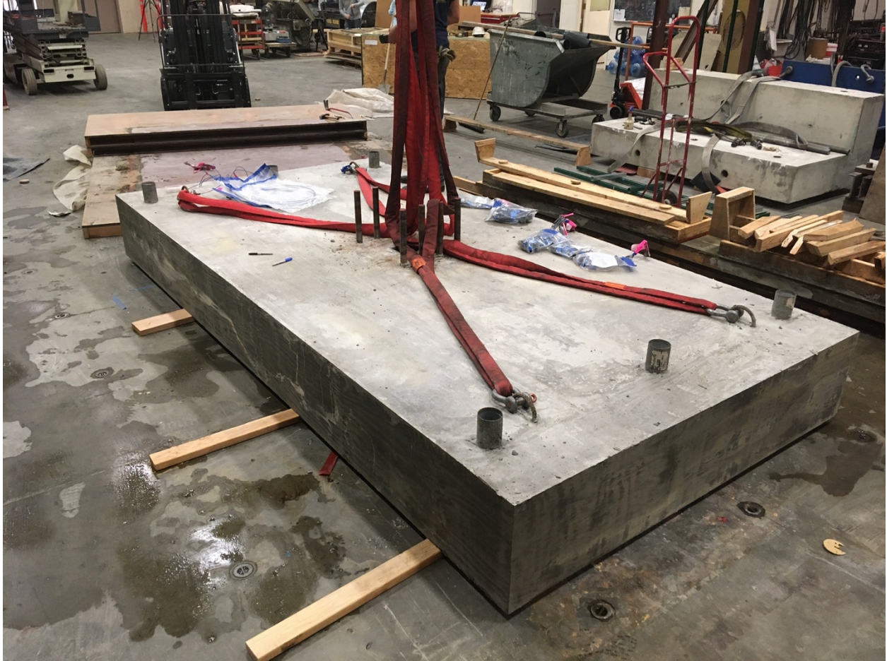
Figure F- 56. Moving specimen with crane
