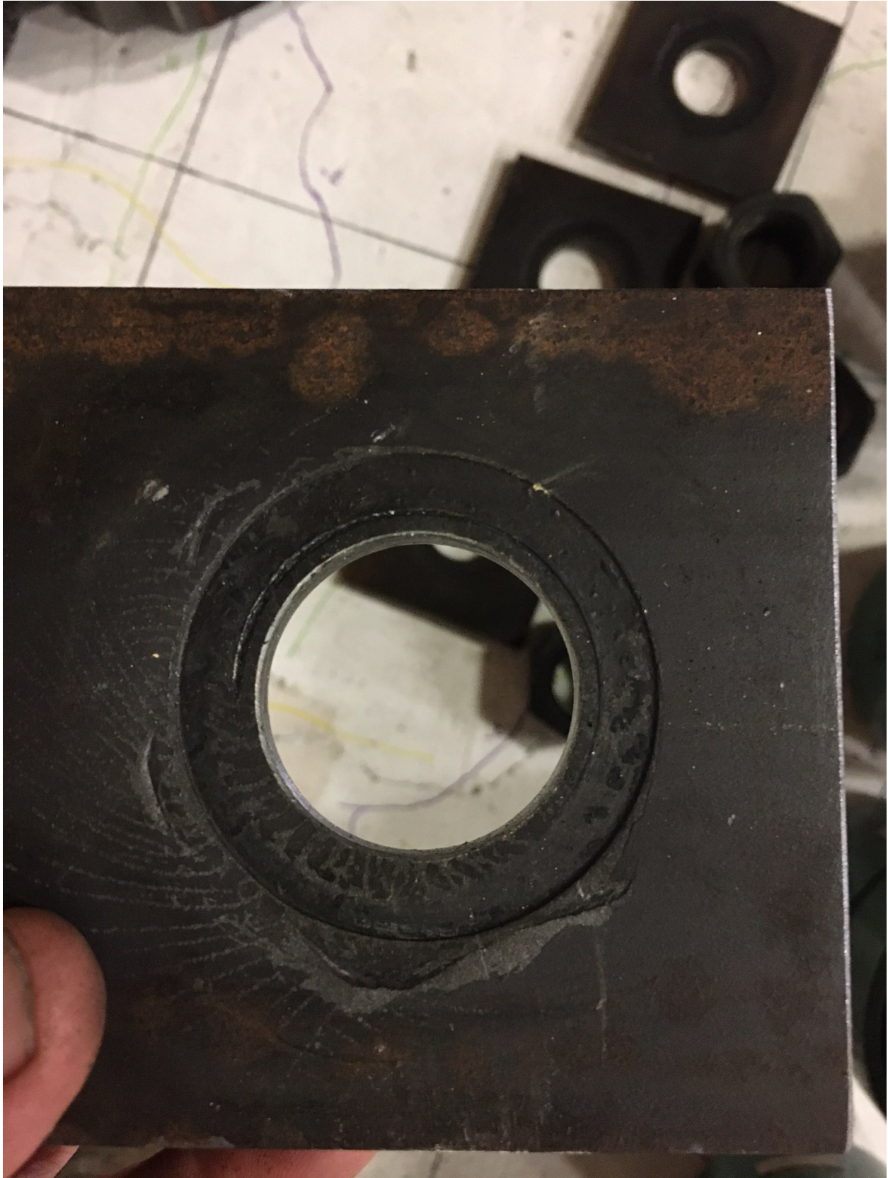
Figure F- 76. Yielding of washers on top of anchor load cells post test
