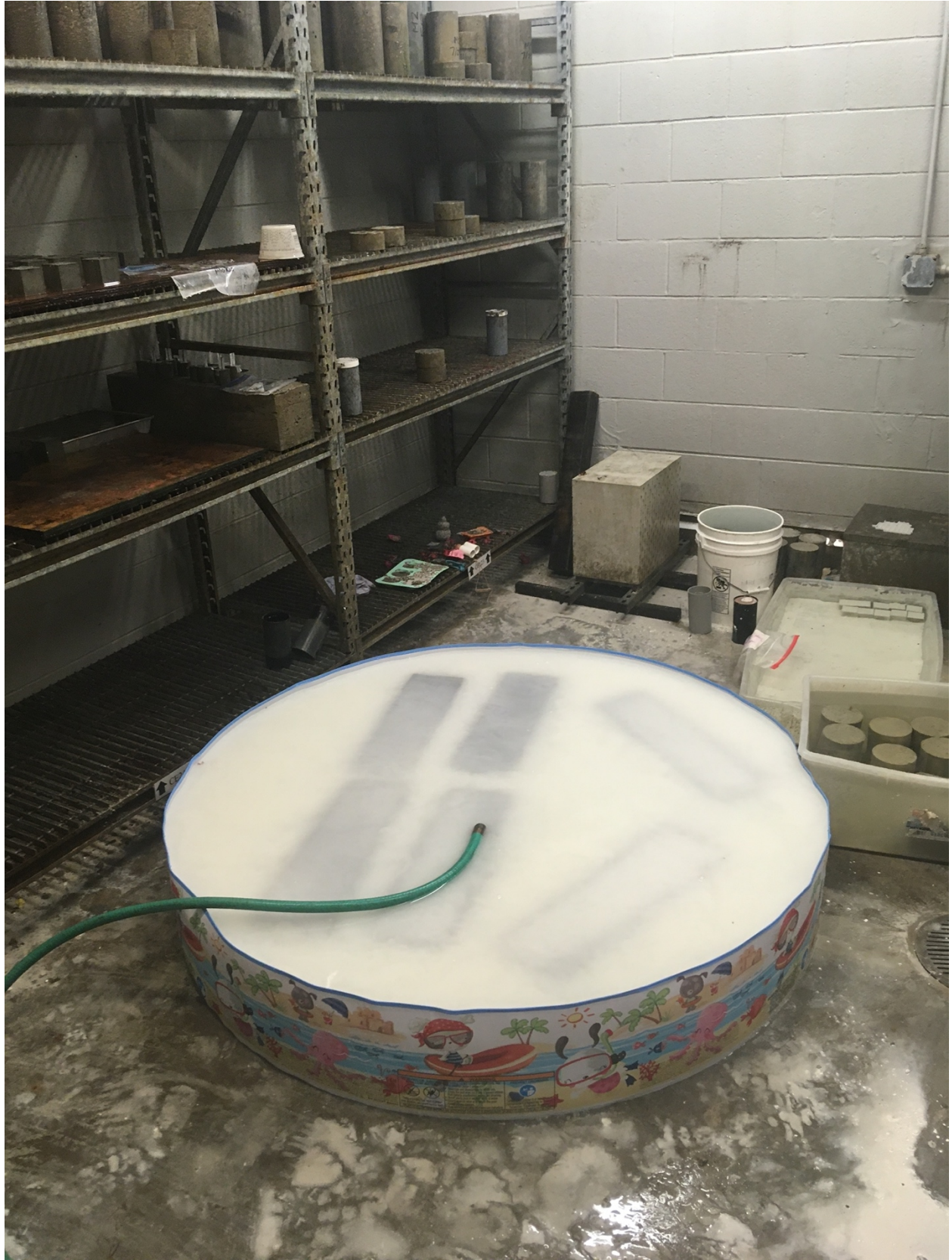
Figure F- 59. Fracture energy beams in lime pool in fog room
