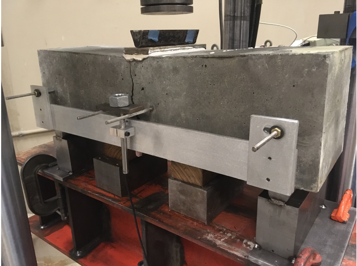
Figure F- 87. Fracture energy tests
