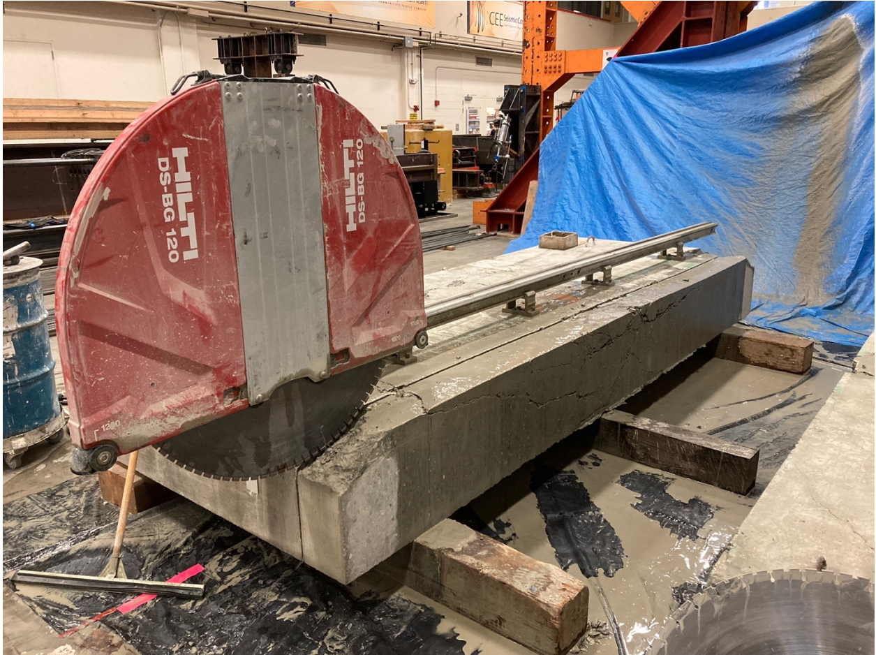
Figure F- 79. Cutting cross sections
