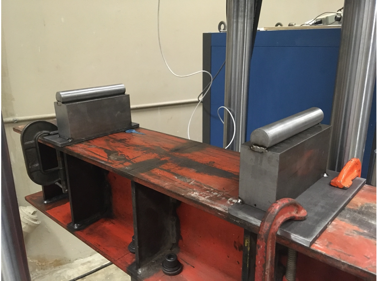
Figure F- 84. Fracture energy tests
