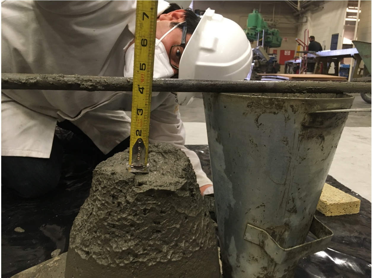
Figure F- 32. Concrete slump test
