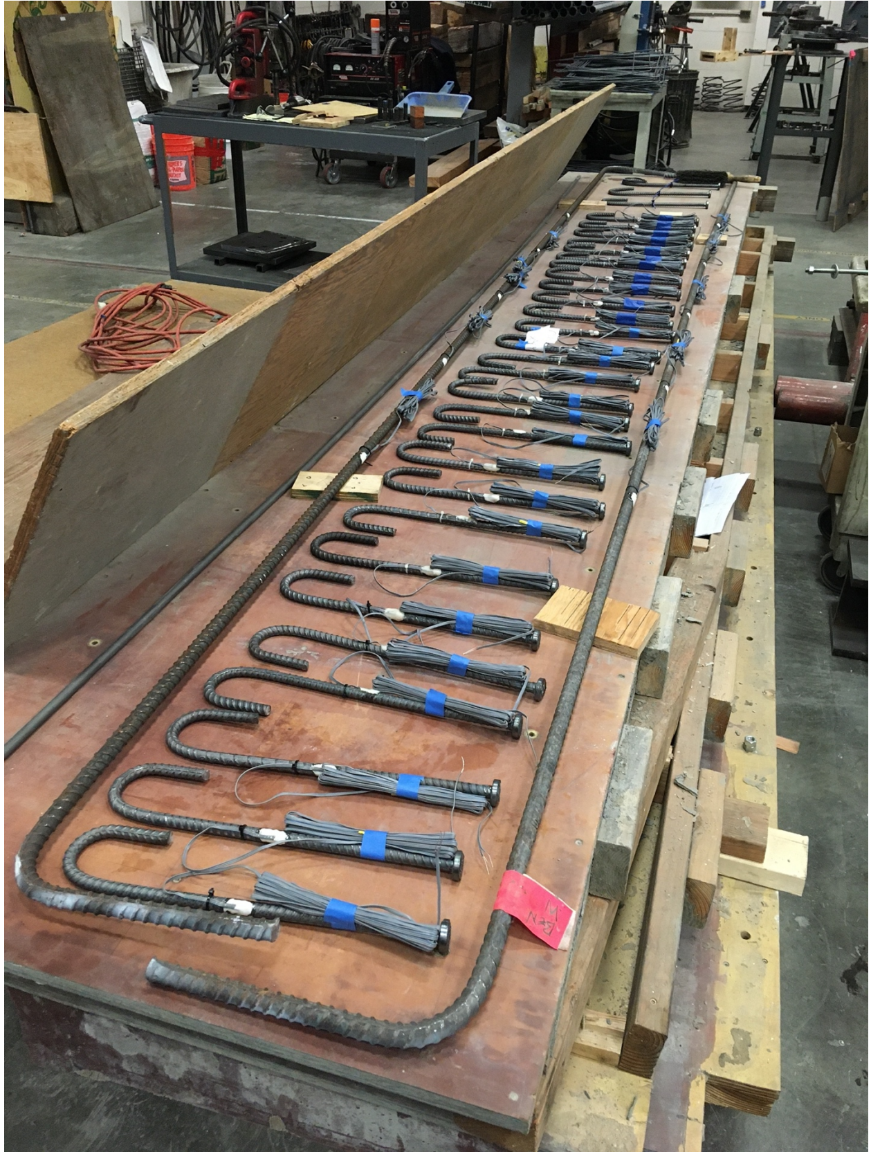
Figure F- 7. Strain gages on reinforcement
