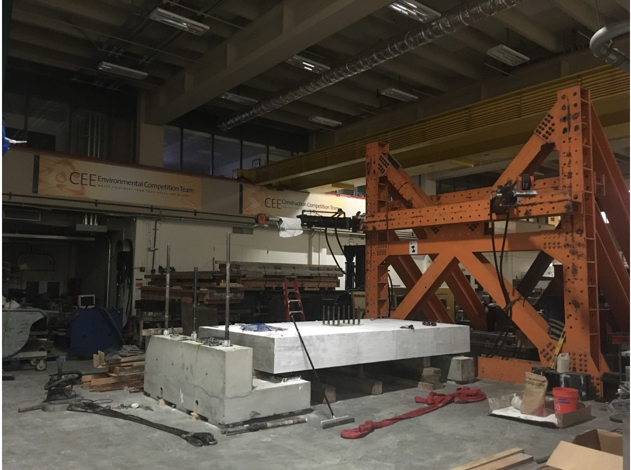
Figure F- 58. Specimen placed on concrete supports
