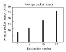
**Fig. 19.** Average latency of AL + XYZ when desitnation number equals to 6, 8, 10, and 12. MUR = 0.3, injection rate = 0.05.
