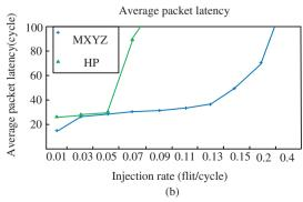
Fig. 15. Comparison of HP and MXYZ in terms of (a) total energy consumption (including both dynamic and leakage power) and (b) latency when MUR = 0.3.
