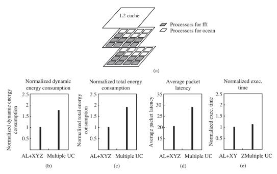
Fig. 21. (a) Two sub-networks in a different NoC architecture. An L2 cache is placed in a separate layer. The other tiles are composed of processors, L1 caches, and routers. Normalized dynamic energy consumption (b), total energy consumption (including both dynamic and leakage power) (c), latency (d), and normalized execution time (e) of AL + XYZ and Multiple UC.
