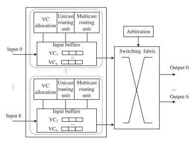
Fig. 3. Router micro-architecture for 3-D NoCs.
