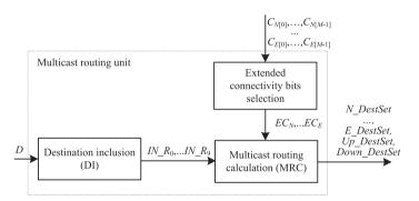
Fig. 13. Structure of the multicast routing unit.
