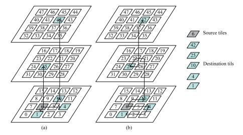
Fig. 7. Comparison of HP and MXYZ in terms of hop counts by an example. (a) The communication paths generated by MXYZ routing. (b) The communication paths generated by HP routing.
