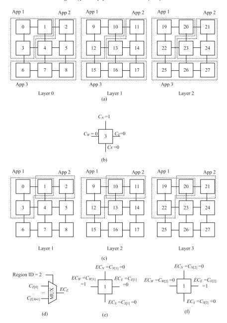
**Fig. 10.** (a) Sub-networks with 3 applications mapped on. (b) Connectivity bits of node 3. (c) Two overlapped sub-networks sharing node 2. (d) Extended connectivity bit generated using a MUX. (e) Extended connectivity bits of node 1 for Sub-network 1 in (c). (f) Extended connectivity bits of node 1 for Sub-network 2 in (c).
