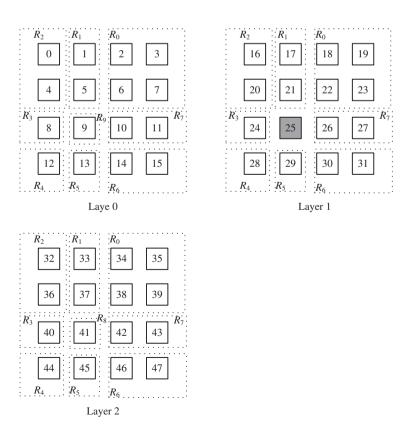
**Fig. 4.** The disjoint regions of tile 25 for a 3-D NoC with  $4 \times 4 \times 3$  nodes.
