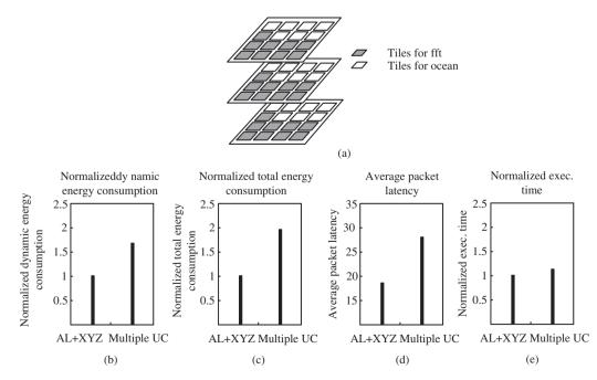
Fig. 20. (a) Two sub-networks in the  $4 \times 4 \times 3$  NoC system. Each tile includes a processor, an L1 I/D cache, an L2 banck, and a router. Normalized dynamic energy consumption (b), total energy consumption (including both dynamic and leakage power) (c), latency (d), and normalized execution time (e) of AL + XYZ and Multiple UC.
