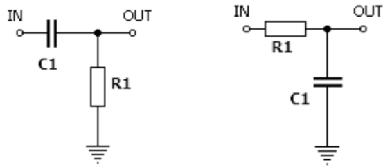
Fig 1.8 High-pass filter and low-pass filter
