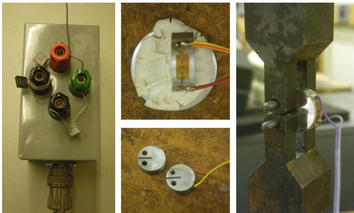
Figure 3.1: Images of sample preparation and mounting in the Instron load frame. Clockwise from left: Wheatstone bridge consisting of three 350 \Omega for signal amplification, sample with attached strain gauge and full wiring, side view of prepared samples, and sample mounted in load frame.
