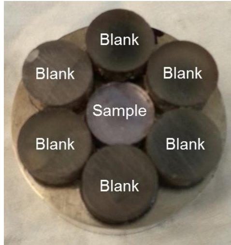
Figure 5.1 – Mounting set up for polycrystalline Y_2O_3 polishing. The sample of interest is in the center
