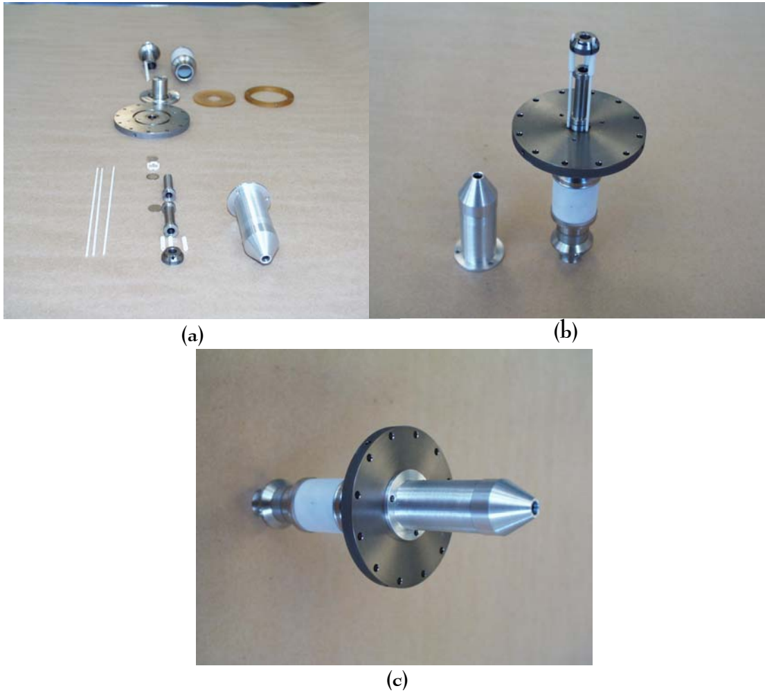
Figure 2.15: Photograph of the ion gun unit. (a) all parts before assembling; (b) configuration of the electrodes assembly without outside housing; (c) whole view of the unit after assembling.
