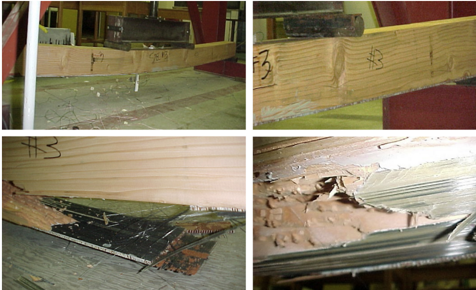
Fig. 17. Ultimate failure of the wood beam strengthened with honeycomb sandwich panel (H-Lam).
