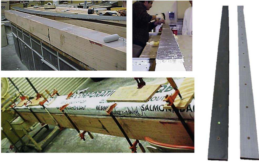
Fig. 4. Application of H-Lam sandwich composites panels on dug-fir beams.
