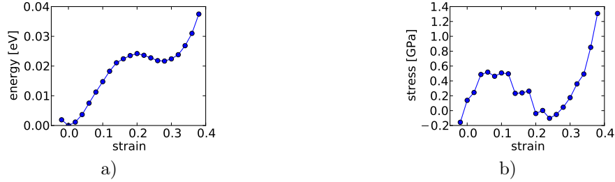
Figure 3.6: The stress-strain and energy-strain relation for the L6 0 structure under a <100> type tensile load. Only the tetragonal path is explored in this simulation. The formation of the FCC phase can be seen at a strain of approximately 25 – 30%. This corresponds to the ordered L1 2 structure.
