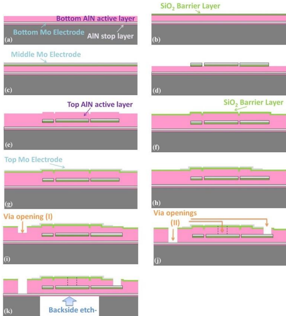
Fig. 3.2.1.1. The process flow of the DEB pMUT: (a) sputtering of AlN/Mo/AlN stack; (b) PECVD SiO 2 deposition; (c) middle Mo Electrode sputtering; (d) patterning of the middle Mo electrode and SiO 2 ; (e) second AlN active layer sputtering; (f) second PECVD SiO 2 deposition; (g) top Mo electrode sputtering; (h) top Mo patterning; (i) via dry etching half-way down to the bottom electrode; (j) via dry and wet etching to expose the middle and bottom electrodes; (k) backside DRIE.
