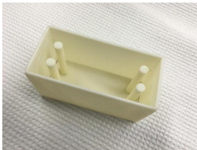
Fig. 5.2.1.1 3D printed mold to make the PDMS samples.
