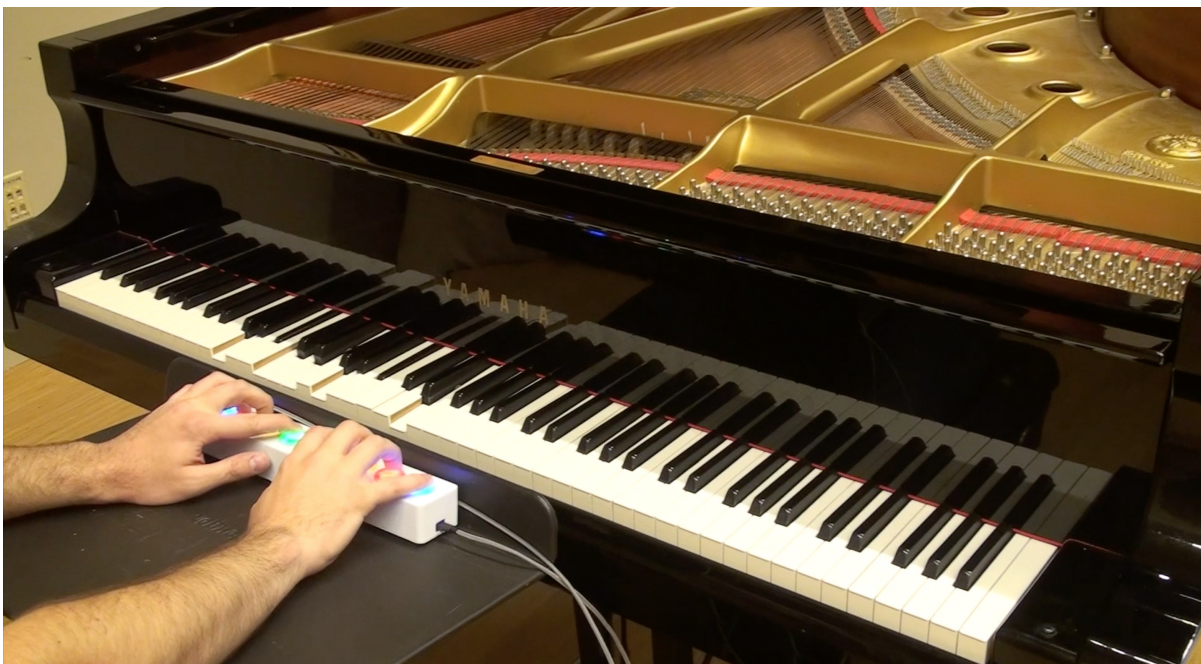
Figure 5.1: Using Piano Genie to improvise on a Disklavier (motorized piano) via MIDI.
