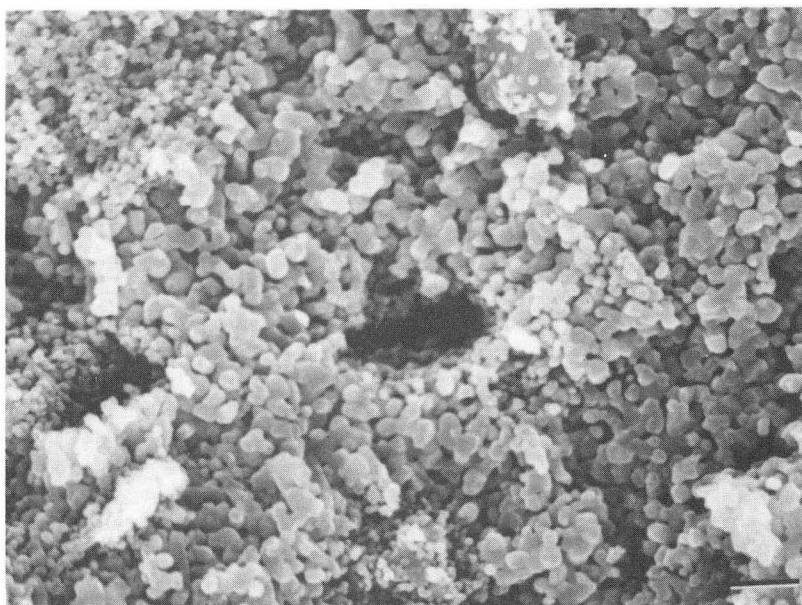
Undoped matrix, 5 vol% SiC, heated to 900 °C.
