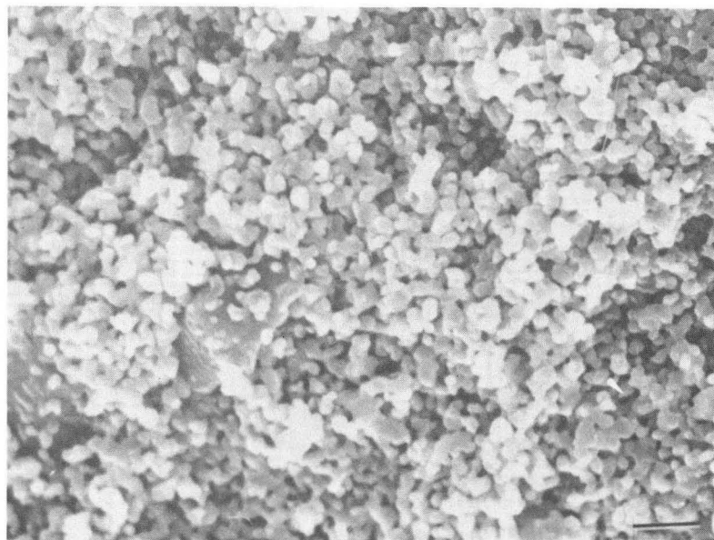
Undoped matrix, 10 vol% SiC, sintered to 1100 °C.
