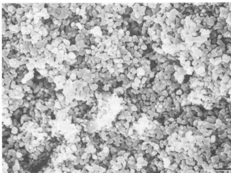
Doped matrix, 5 vol% SiC, heated to 900 °C.
