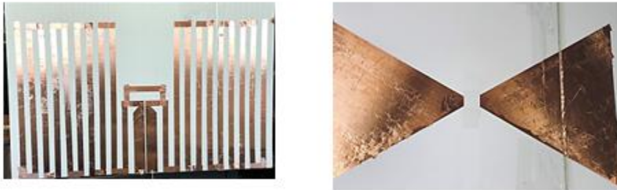
Figure 4.9. Fabricated antennas for measurement setup. Self-resonance antenna (Left). Unmatched electrically small bowtie antenna (Right)
