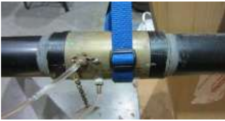
Figure 5: 2-685 Gerand venturi low-flow reference meter mounted in measurement apparatus
