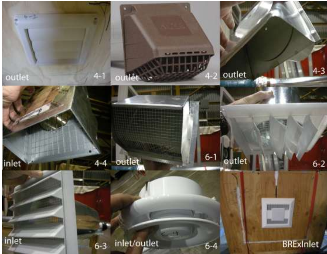
Figure 8: Terminals used for laboratory measurement. The first number in bottom right of each image indicates the diameter of the terminal’s duct connection in inches. The BRExInlet has a four-inch diameter connection.
