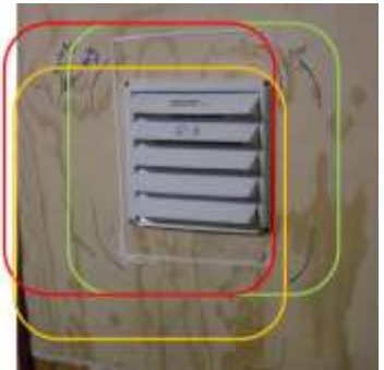
Figure 9: The three locations: middle (green), edge (red), and corner (yellow) of the terminal relative to the face of the flow hood
