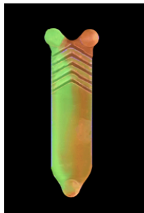
Figure 9. Enhancing mixer functionality by adding grooves
