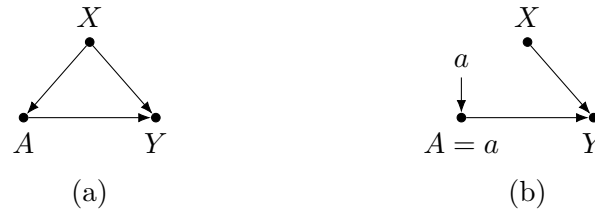
Figure 13. Backdoor criterion: (a) unmodified causal graph where A affects Y , and X represents the covariate set of variables selected for adjustment; (b) modified causal graph where for everyone in the population X is set to x . This is do -calculus, and is used to derive an adjustment formula.
