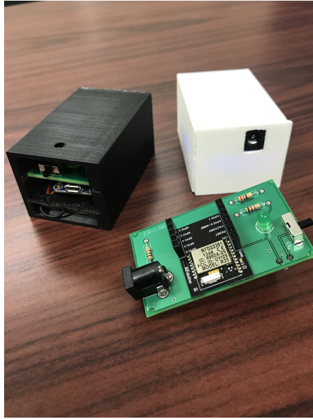
Figure 3.8: Jump receiver box built with an RFduino
