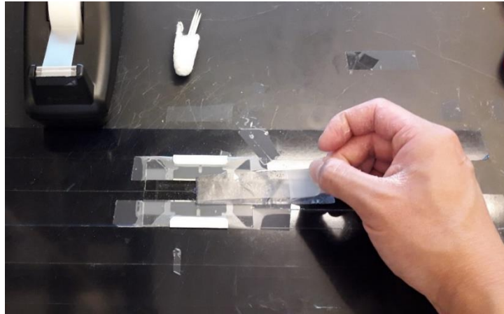
Figure 3.4 Exfoliation by Peeling. Tape is peeled off in a smooth and steady manner to leave behind ultrathin flakes of the desired material.
