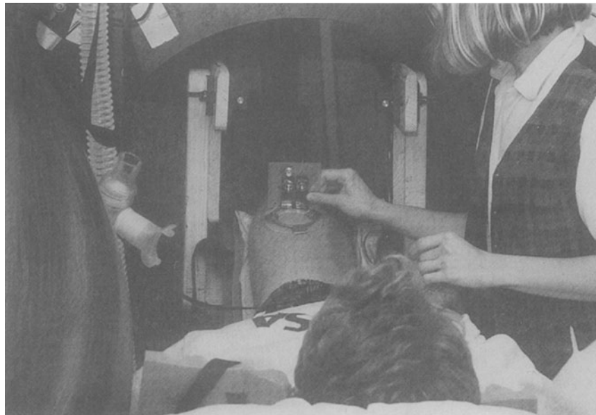
Fig. 8.6. Application of a surface coil to Russ Richardson (University of California, San Diego) by Liz Noyszewski for NMR studies of muscle oxygenation at the University of Pennsylvania. Note equipment for pulmonary gas-exchange measurements (left), ergometer support flanking coil, and magnet in background. Courtesy of R. Richardson and P.D. Wagner (see ref. 137).
