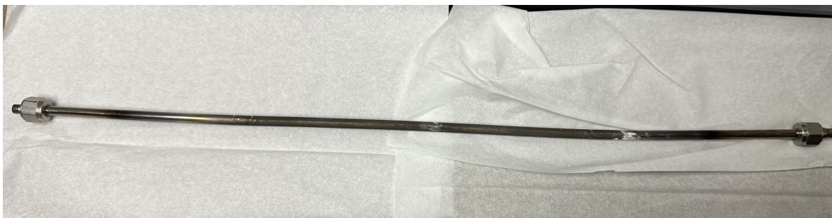
Figure 7.4: FeCrAl alloy tube after first oxidation procedure at 950 °C for 10 hours.
