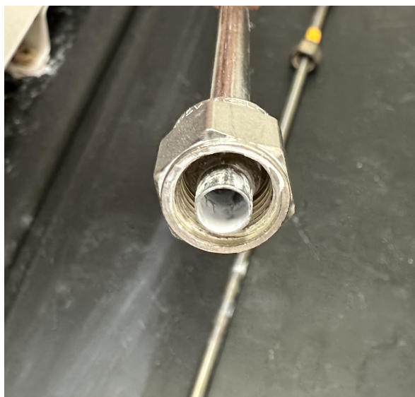
Figure 7.6: Wet \text{ZrO}_2 washcoat monolith at the end of FeCrAlloy reformer tube prior to calcination and Ni catalyst embedment.
