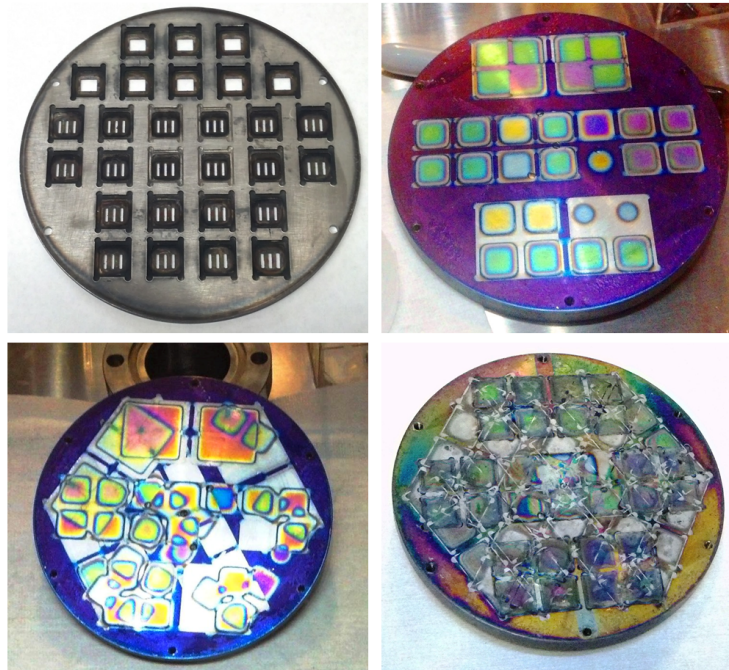
Figure 2.4: Shadow mask for sputter deposition and resulting quasi-random patterns on the backing plate. The top left image shows one of the shadow masks used for sputter deposition. It is machined from stainless steel to hold 28 (glass) substrates of 12 x 12 mm size. The other images shows patterns found on the backing plate of the substrate holder after several deposition runs with different patterns.
