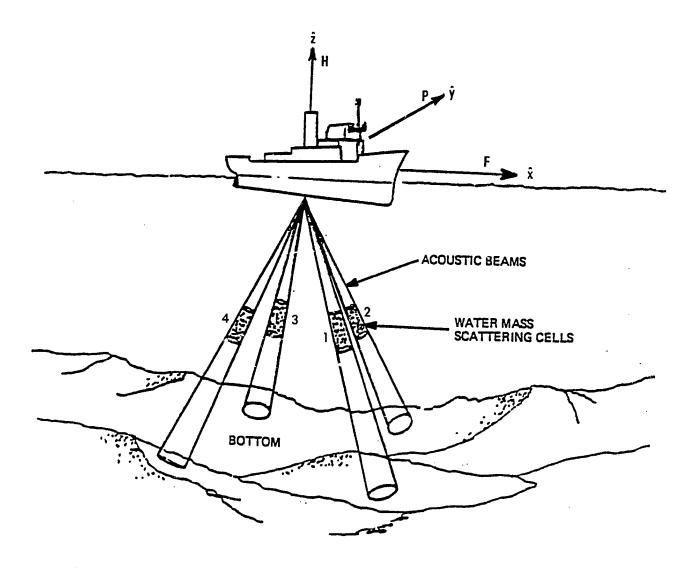
Fig 2.2: Range Gated Shipboard Doppler System. Four beams (fore, aft, port and starboard) equally inclined from the ship's vertical axis acoustically probe the ocean. The Doppler shift in backscattered signal measures the relative velocity between ship and ocean. Range gating allows depth profiling of currents.
