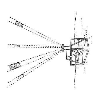
?ig. 2.3: A Doppler current profiler which has been bottom mounted for vertical profiling of local currents.
