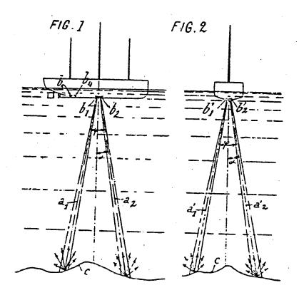
Fig. 2.1: The use of acoustic Doppler shift to measure the velocity of ships at sea dates back to this patent by C. Chilowski, submitted in 1924. Note the sophisticated 4 beam Janus design which is still used for first order pitch and roll compensation.
