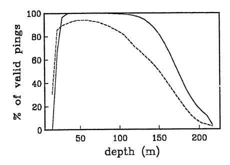
Fig 3.1: Depth range of shipboard measurements is shown by the percent of pings for which the profiler electronics indicated valid returns at each range bin. Two 12 hour subsets of data are shown, one each from 1981 and 1982. Details of such validity profiles vary with many factors including location and time of day.
