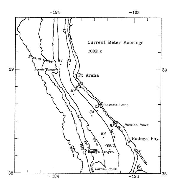
Fig. 5.1: CODE 2 (1982) moored current meter array. Table 5.1 provides details on instrumentation at each mooring. Also shown is the location of wind buoy NDBO 46013.
