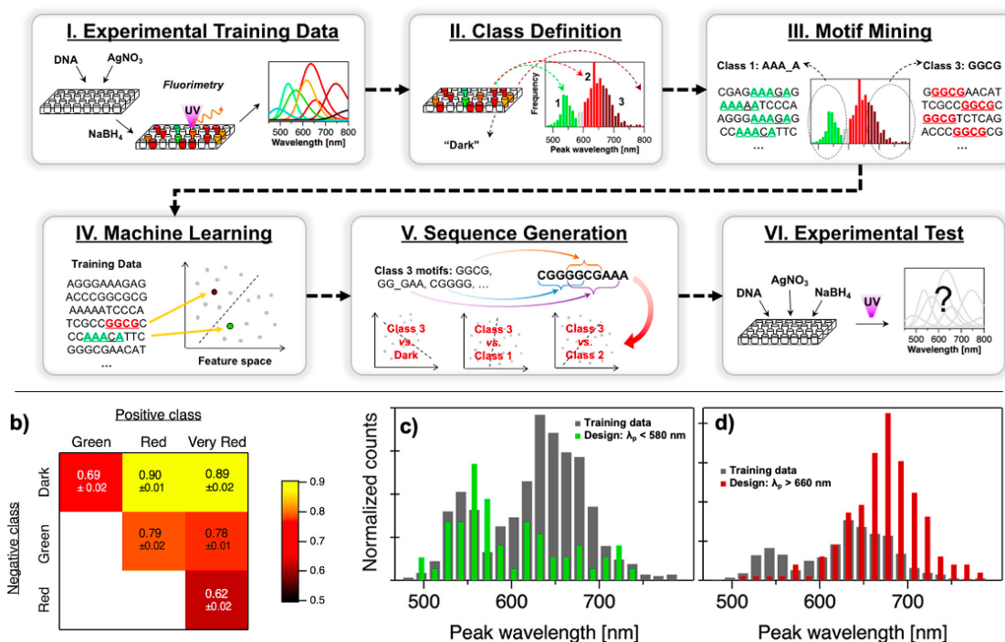
Fig. 7 ML-guided design of \text{Ag}_N -DNAs with fluorescence emission in specific spectral windows. 71 a) Schematic of ML workflow. b) Cross-validation scores of one-versus-one SVMs for each color class pair. c,d) Adapted from Copp, et al. , 71 with permission from the American Chemical Society. Copyright 2018.
